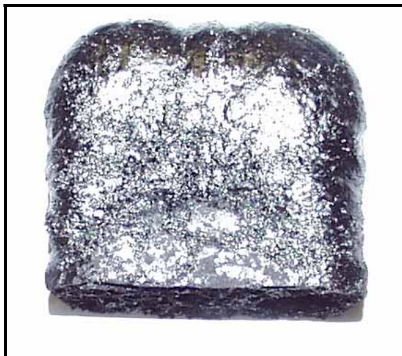
Figure 6. Foam made from 185 °C softening point pitch
