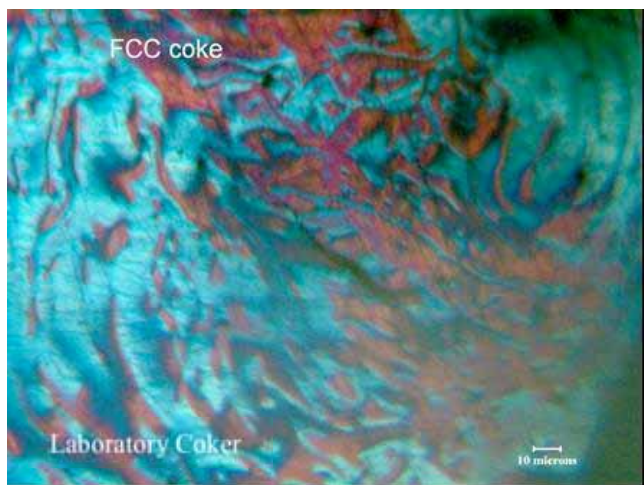
Figure 9 FCC Calcined Coke from Laboratory & Delayed Coker
