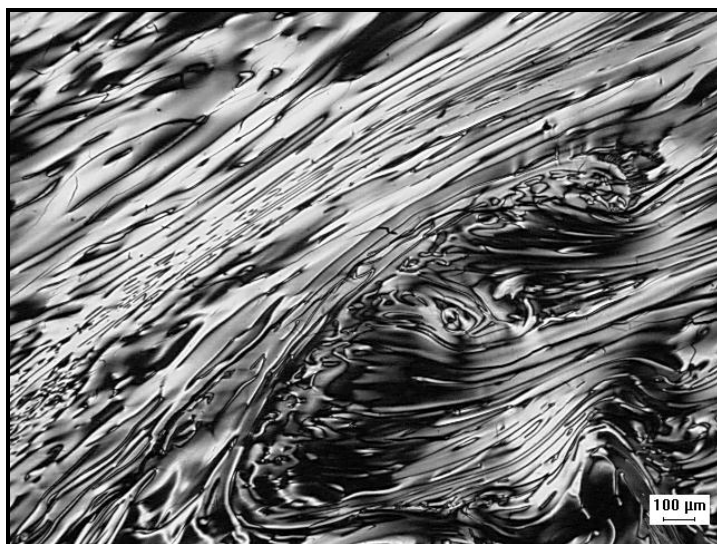
Figure 8: Polarized Light Micrograph of a Predominantly Flow Oriented Region in the Bottom Sample from Coke Run 1 with Seadrift Decant Oil
