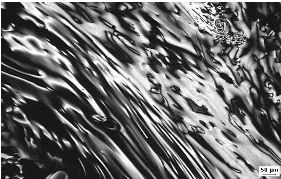
Figure 12b: Polarized Light Photomicrograph Showing Well-Oriented Coke in the Top Region of Coke Obtained from Run 3 with CTD at 50 psig.
