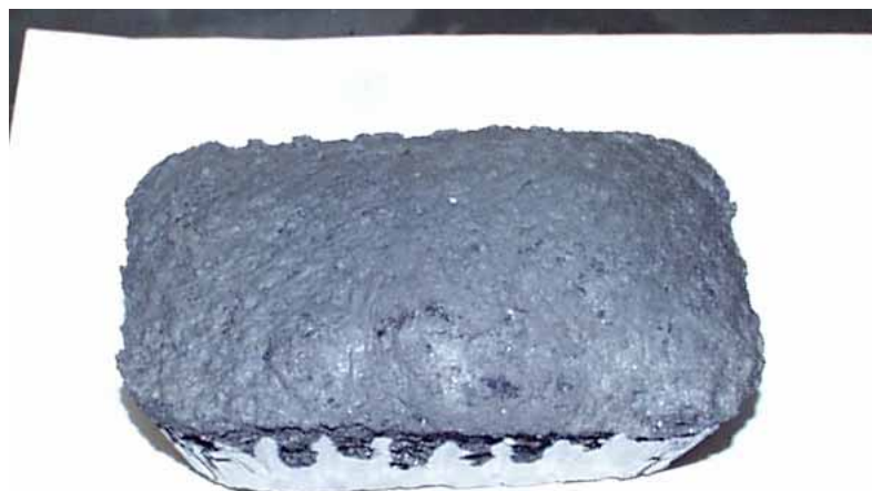
Figure 7. Foam made from devolatilized binder pitch
