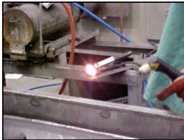
Figure 4. Close-up of the carbon sample, still glowing white hot after the torch is removed. Plasma torches are able to cut through steel in seconds, but carbon foam is able to resist cutting for several minutes.
