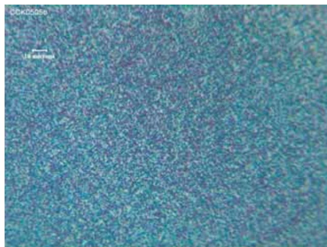
Figure 7 Anthracene Oil derived Coal Extract Coke - Small Mozaic Anisotropy
