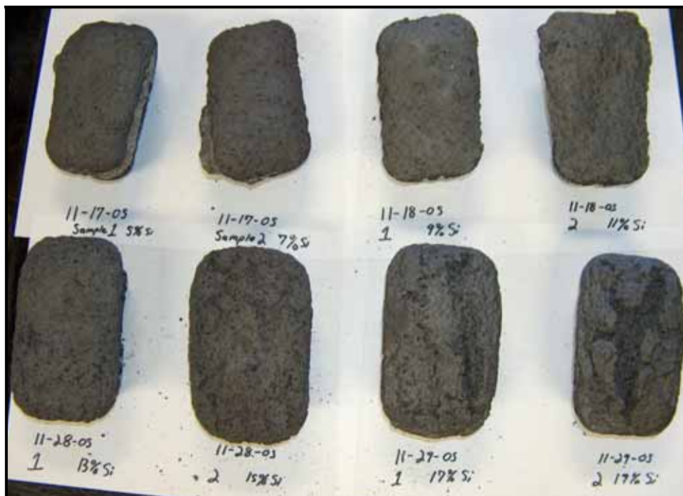
Figure 8. Samples containing from 5 % to 19 % \text{SiO}_2 .
