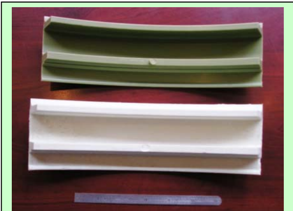
Patterns of Shroud Liner Made from FOPAT (white) and Wax (green)
