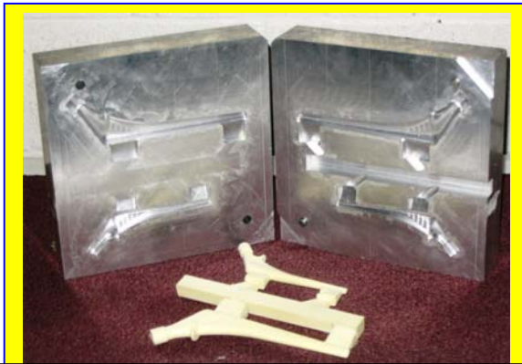
Photo #1 GE/AF SUPPLIER Provided Pattern Injection Die
