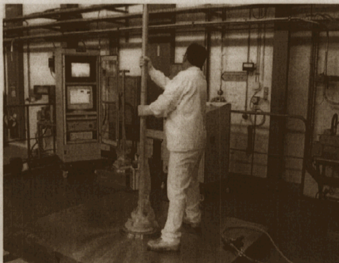
Fig. 2. Operators pumping sludge at Marcoule required little protective equipment. (Ref. 6)
