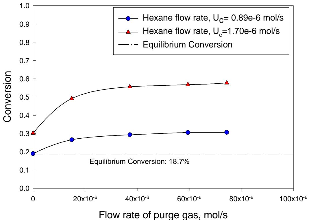
Figure 1: Dehydrogenation of cyclohexane in Pd-ceramic membrane reactor
