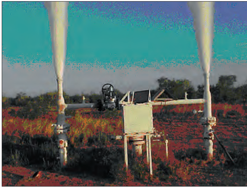
Figure 6.2. CO 2 venting during pipeline purging
