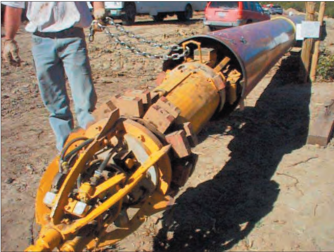
Figure C1.20. Lineup clamp shoes for pipe joint
