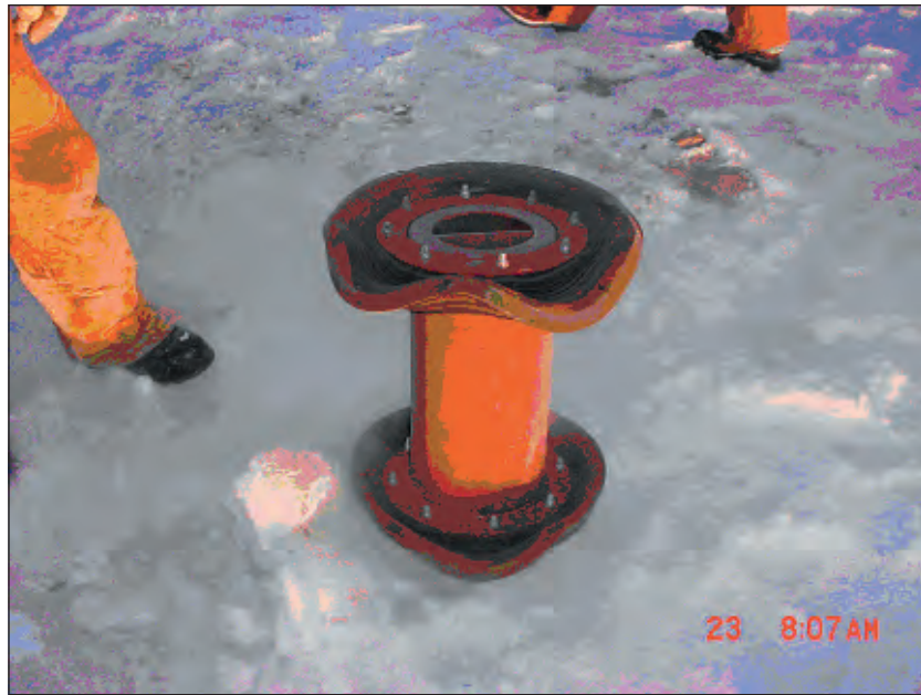
Figure 6.4. Pig damage from depressuring too rapidly
