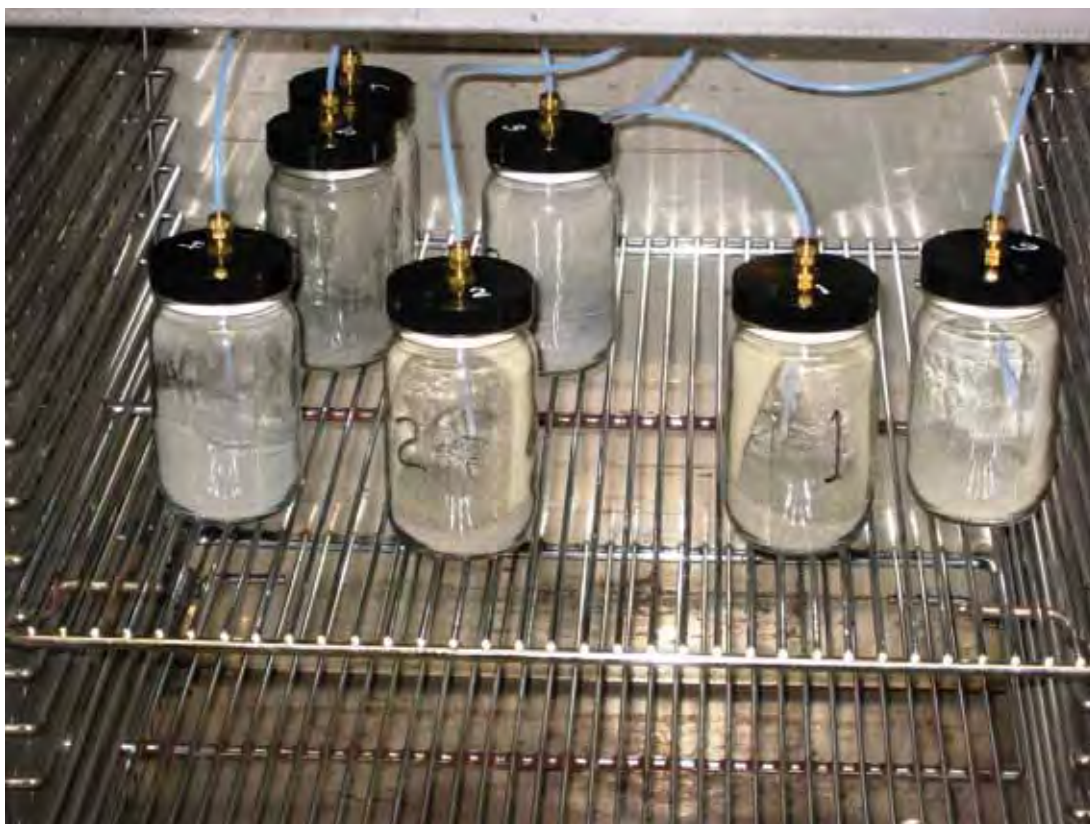
Figure 52. Mercury Volatility Fly Ash Samples in 140 °F Oven
