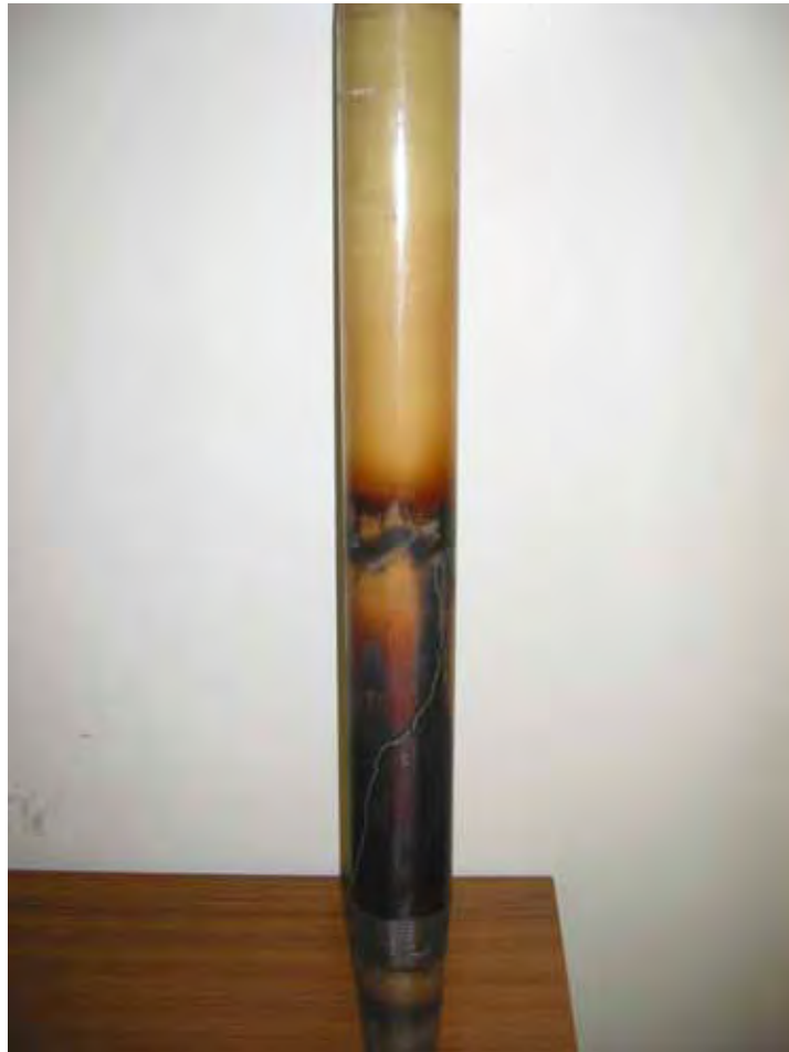
Figure 50. Failed High-Voltage Rapper Rod Insulator, Lower Portion Blackened by Acid Condensation
