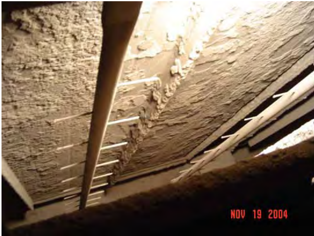
Figure 16. Fly Ash Accumulation on Pilot ESP Collector Plate, Field #1
