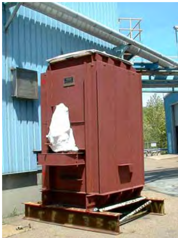
Photo 3-B. Ljungstrom-Type Pilot Air Heater (Before Installation)
