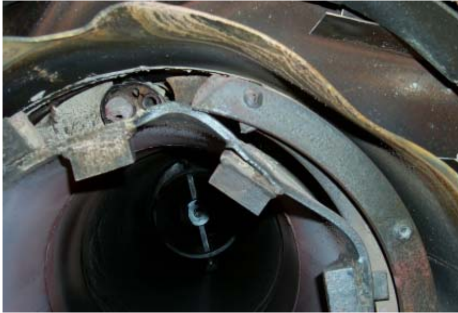
Figure 53 – Example of Overheat Damage on Modified Burner
