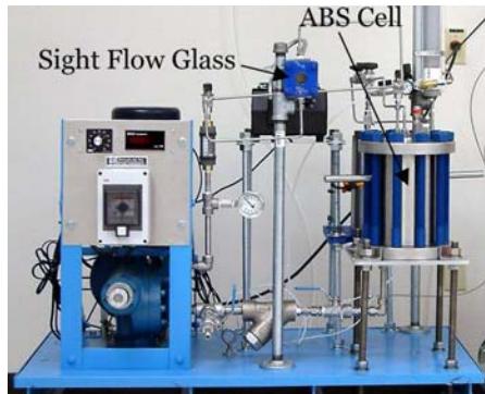
Figure 1: HTHP Re-Circulating System with Acoustic Bubble Spectrometer, 3 in. x 3 in. Hydrophones & Visual Monitoring Equipment
