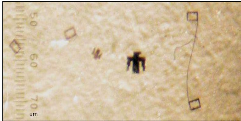
Figure 4.3.1-3: Optical images of Several MEMS samples from SNL, shown with a micron scale on the left.
