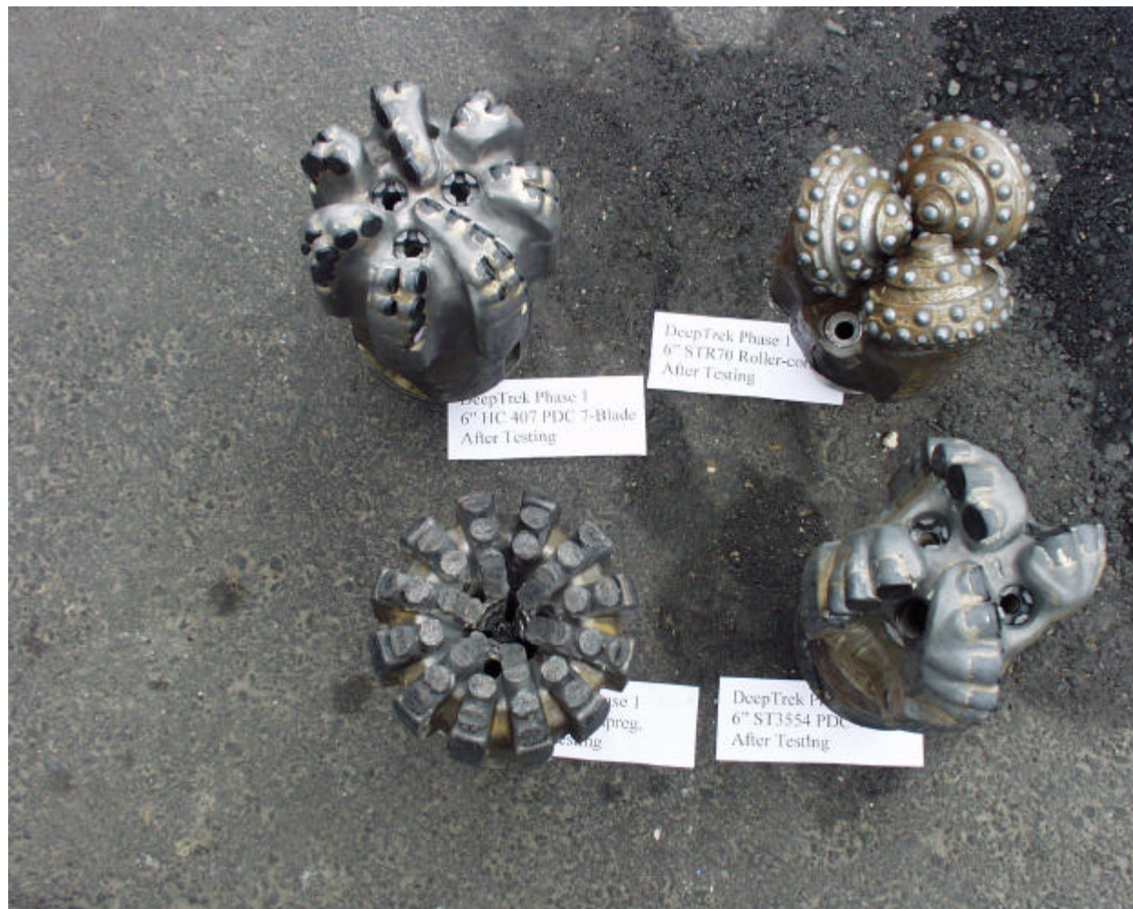
Figure 4. Hughes Christensen Drill Bits Used in DeepTrek Tests
