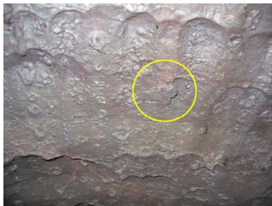
Figure 2. Slagging gasifier refractory sidewall showing corrosive wear and with spalled material (circled).
