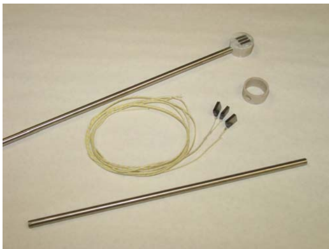
Figure 2 – A completed high temperature corrosion rate probe and the components of construction.
