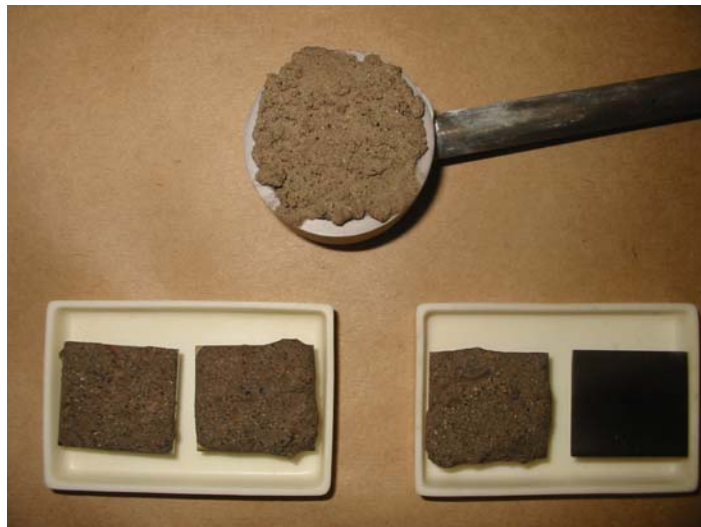
Figure 3 – Electrochemical corrosion rate probe and mass loss coupons prior to testing but after the application of a layer of ash. One coupon (far right) intentionally ash free.
