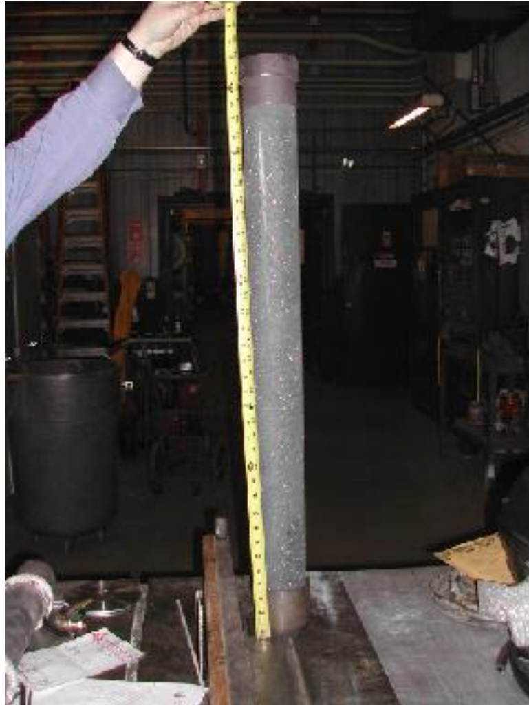
Figure 62. Silicon carbide indirect air-cooled liner with transition pieces
