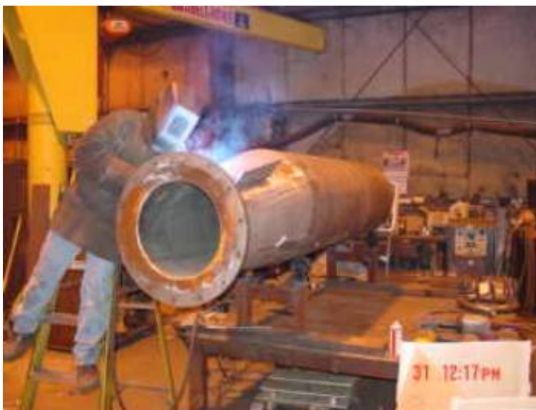
Figure 71. PREHEAT combustor shell during fabrication
