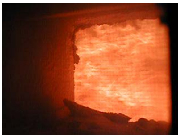
Figure 43. Modified burner, flame roots are more uniform
