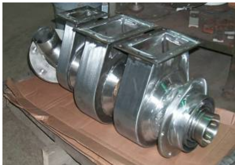
Figure 35. Original PC burner used for pilot-scale PC PREHEAT testing
