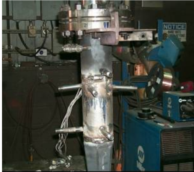
Figure 34. Modified gas-fired combustor for pilot scale testing
