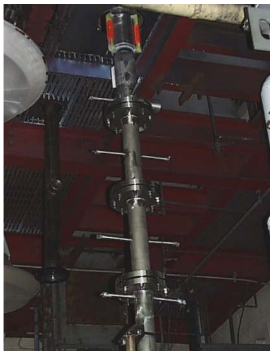
Figure 19. Variable length preheating chamber permits testing with various preheating residence times
