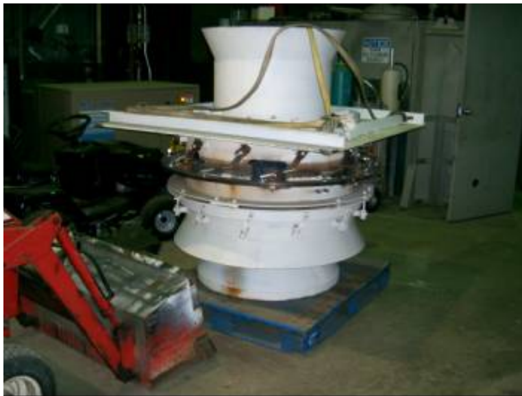
Figure 70. CCV burner during PREHEAT modifications
