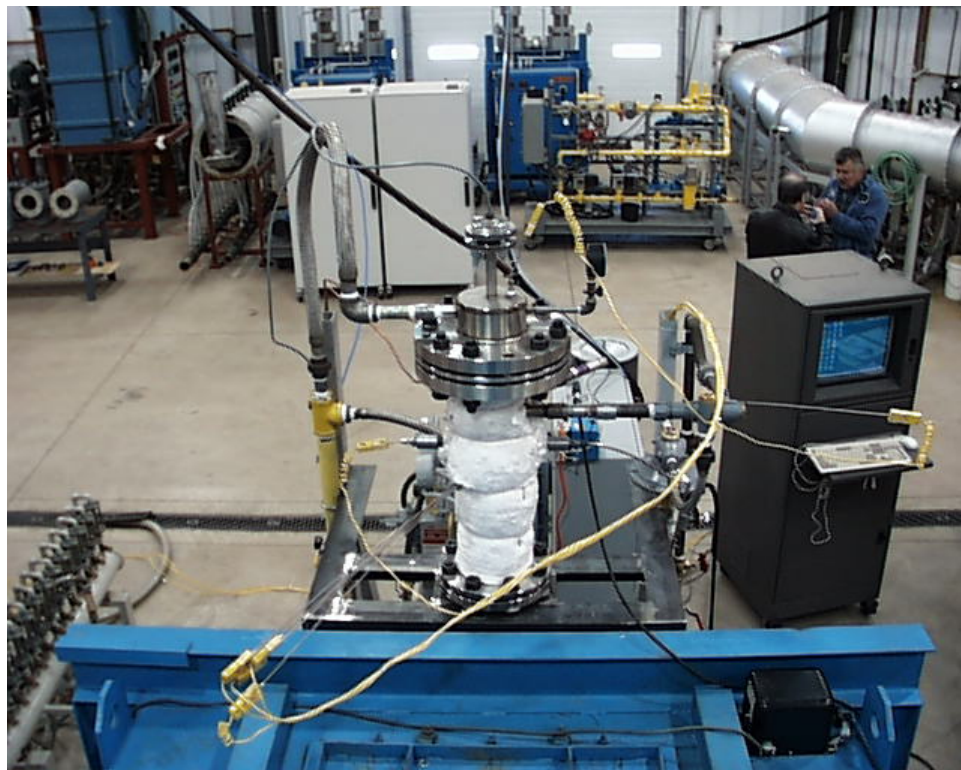
Figure 17. PC PREHEAT combustor unit - view from the top of the sectional furnace
