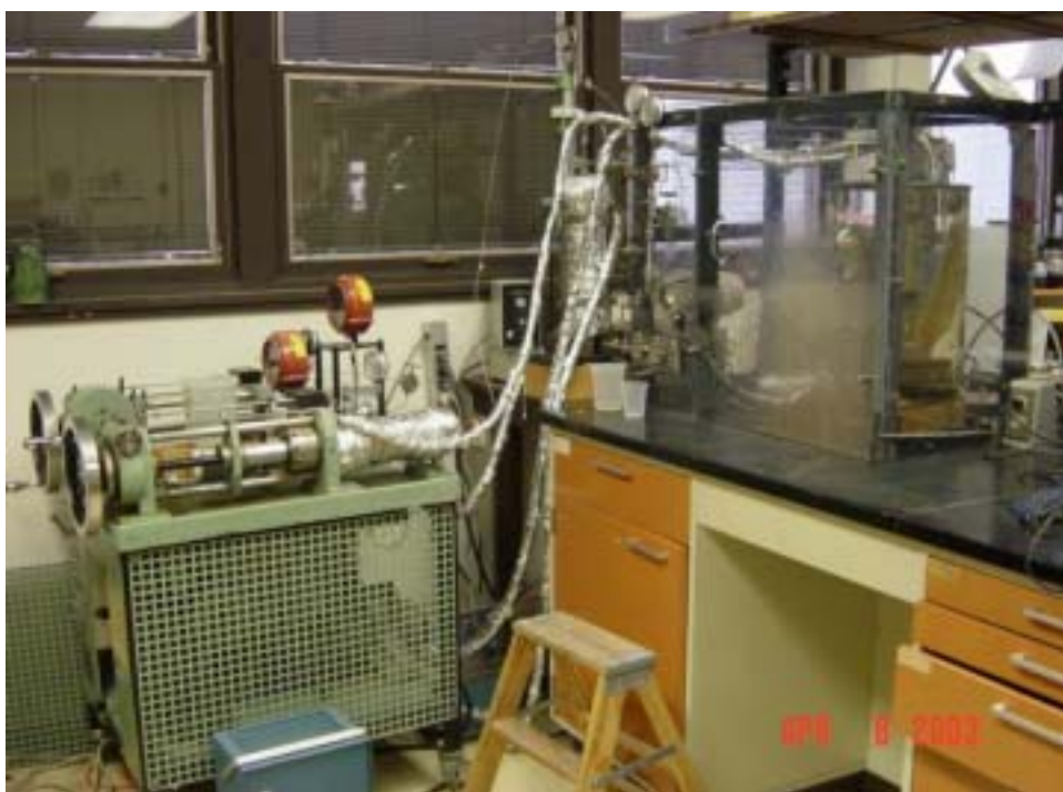
Fig. 1-6. Foam stability apparatus setup.
