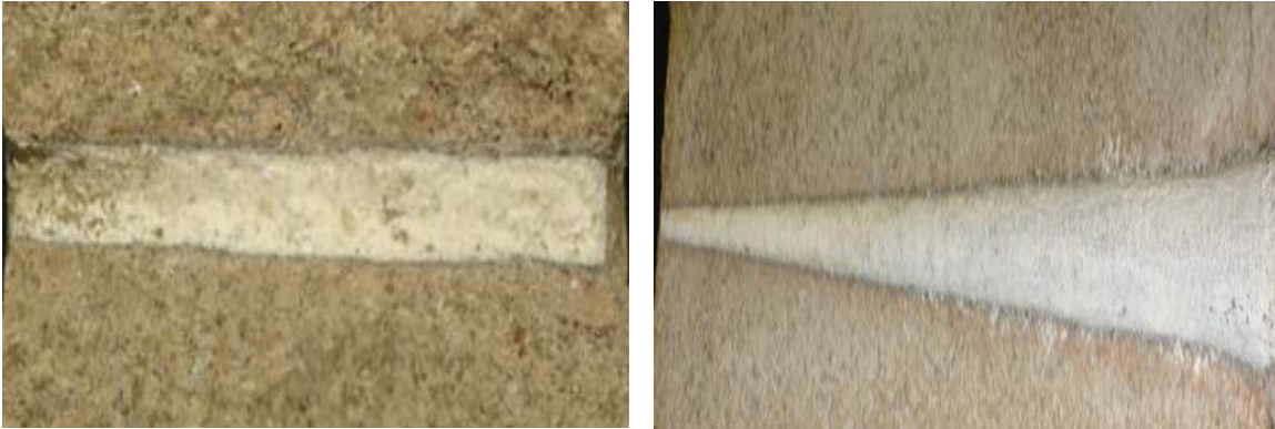
Figure 18. Different hole geometry produced by shaping laser beam with different lenses
