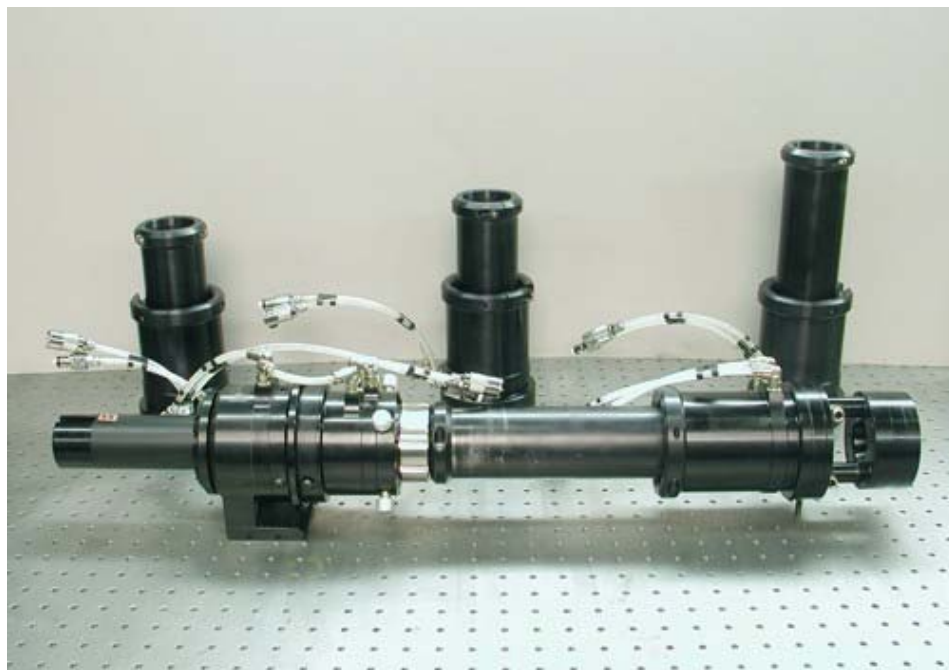
Figure 66. Collimator for HPFL provides beam from 6.35 mm (0.25 in) to 2.54 cm (1.0 in) diameter
