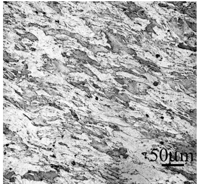
Figure 7. Cross-sectional view of a) as -received, recrystallized and b) cross-rolled and recrystallized MA956 tube ( \beta=8^\circ ). The grain shape is significantly modified, with the long axis now stretched along the hoop direction.
