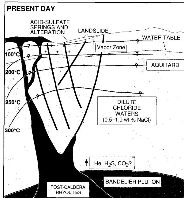
Samples taken from this corehole indicate that the fluid column in the upper part of the corehole had boiled. Nowhere before has such a detailed suite of samples been obtained throughout the boiling interface in a geothermal well. Fluid inclusion data indicate that the hydrothermal system has boiled intermittently throughout its history to depths
