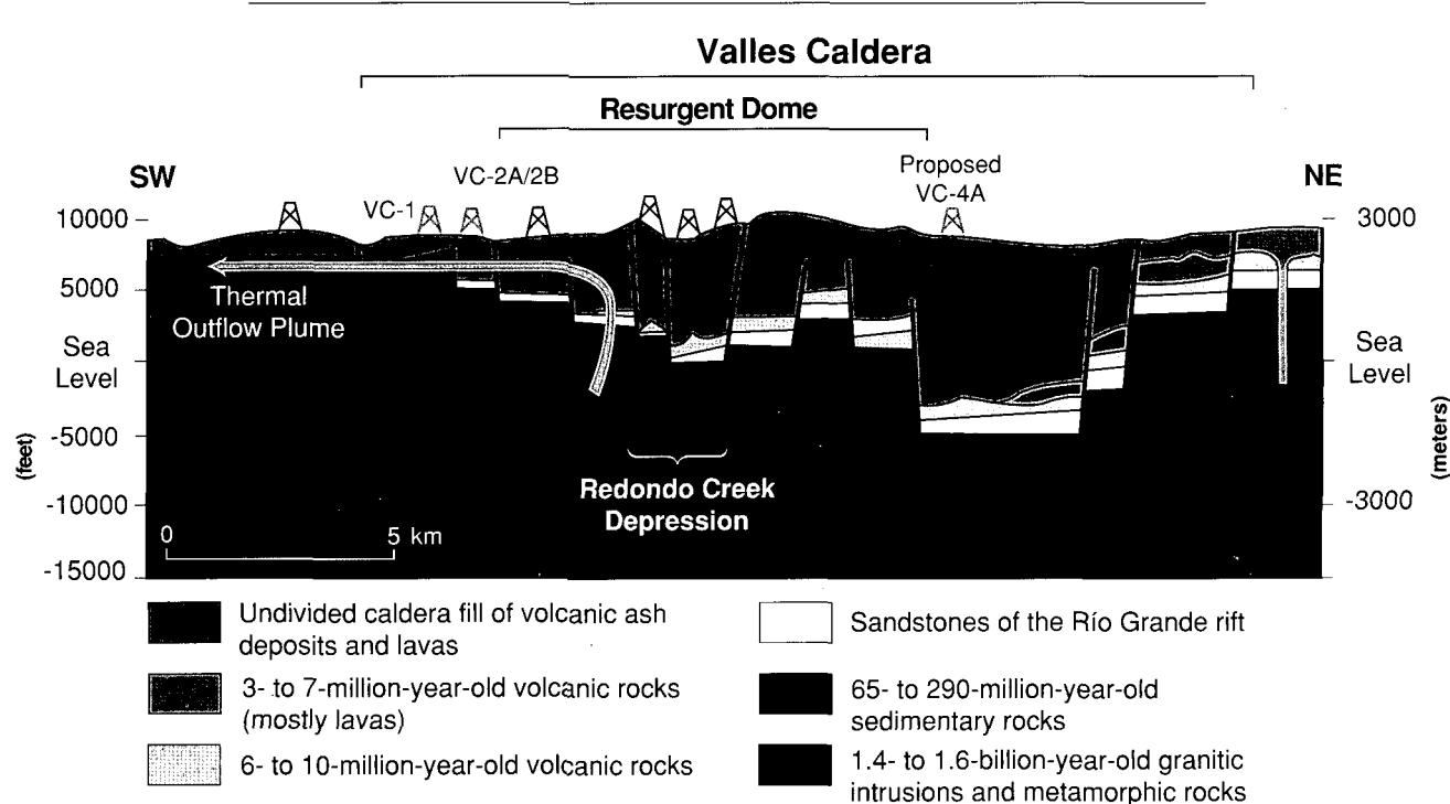
*A cross-section of the Jemez volcanic field and Valles caldera showing the strata and their depths. Temperatures within the caldera are as high as 648°F, which is an indication of the youth of this volcanic field and its active geothermal systems. The western margin of the Río Grande Rift, a major north-south depression that divides New Mexico, underlies the Valles caldera.*
