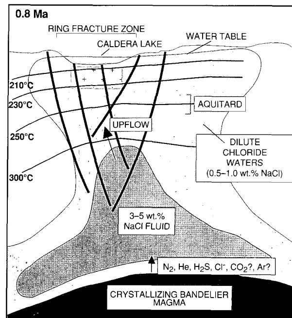
*This conceptual shows the possible evolution of the western half of the Valles caldera subsystem between 0.8 Ma and the present. The aquitard is now 900 m below surface level, and the water table lies approximately 250 m below the surface. (The open stipple pattern denotes high-level molybdenite mineralization.)*
