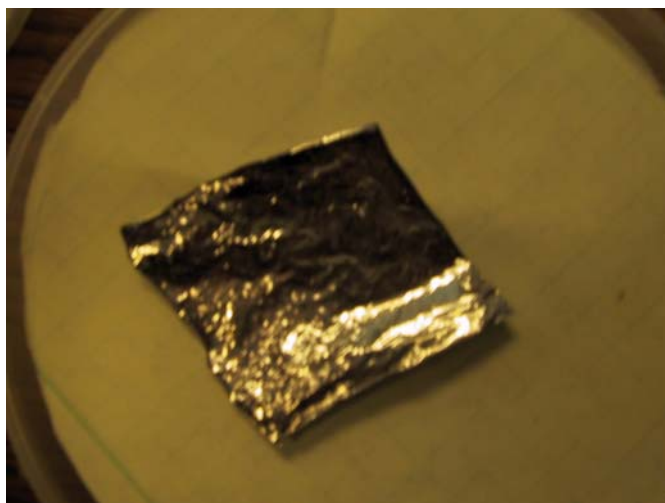
Figure 3. Sample 073106#1 after 24 hours at 400 °C in forming gas
