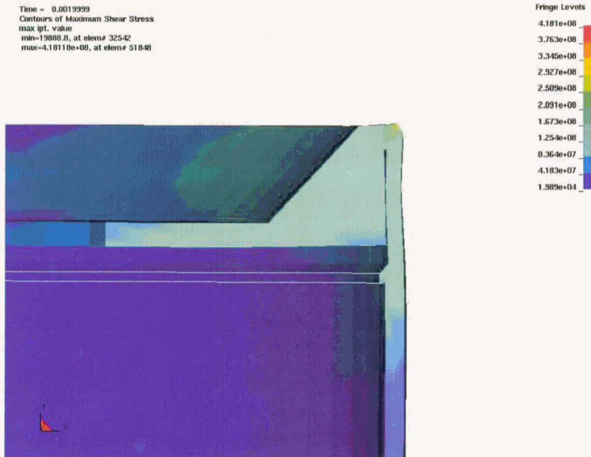
Figure 11. Outer Shell Maximum Stresses at 600 °F Using Vendor Elongation
