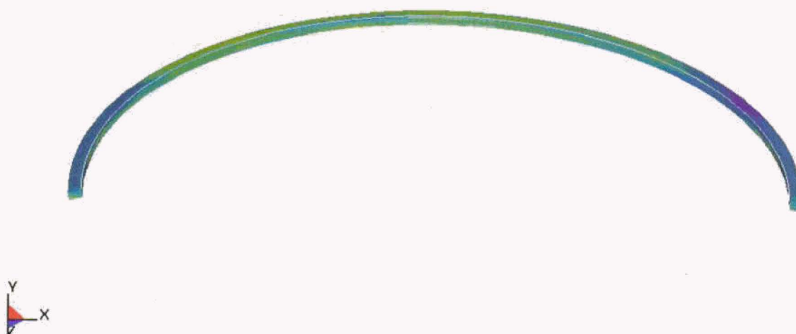
Figure 14. Shear Ring Stresses at 600 °F
