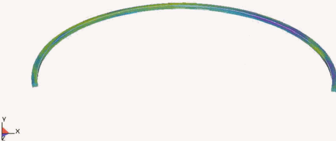
Figure 13. Shear Ring Stresses at 400 °F
