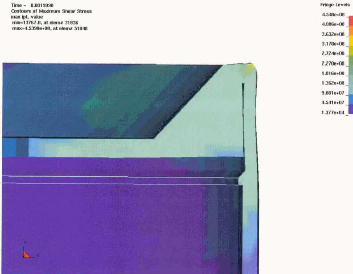
Figure 9. Outer Shell Stresses at 400 °F
