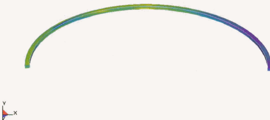
Figure 12. Shear Ring Stresses at Room Temperature
