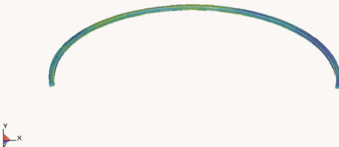
Figure 15. Shear Ring Stresses at 600 °F Using Vendor Elongation
