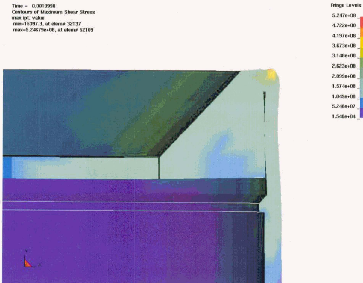
Figure 8. Outer Shell Stresses at Room Temperature
