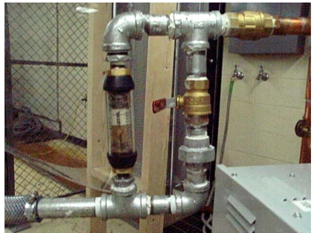
Figure 7. Photographs of parts of the Dimpled Tube Heat Exchanger Test Facility, including: (a) the water heating device, (b) the total pressure probe and wall static pressure tap, and (c) the rotameter used to measure the water volumetric flow rate.
