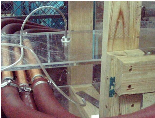
Figure 7. Photographs of parts of the Dimpled Tube Heat Exchanger Test Facility, including: (a) the water heating device, (b) the total pressure probe and wall static pressure tap, and (c) the rotameter used to measure the water volumetric flow rate.
