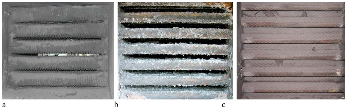
Figure 29. Visual State of the Test Sections Internals After the Trial: a -finned, b - dimpled (in-line arrangement), c - dimpled (staggered arrangement)
