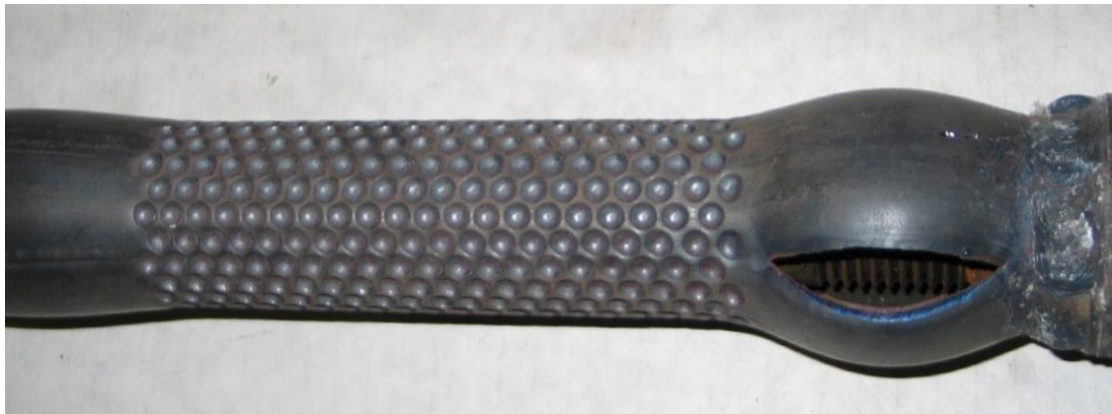
Figure 5. Dimpled tube sample after "burst" test
