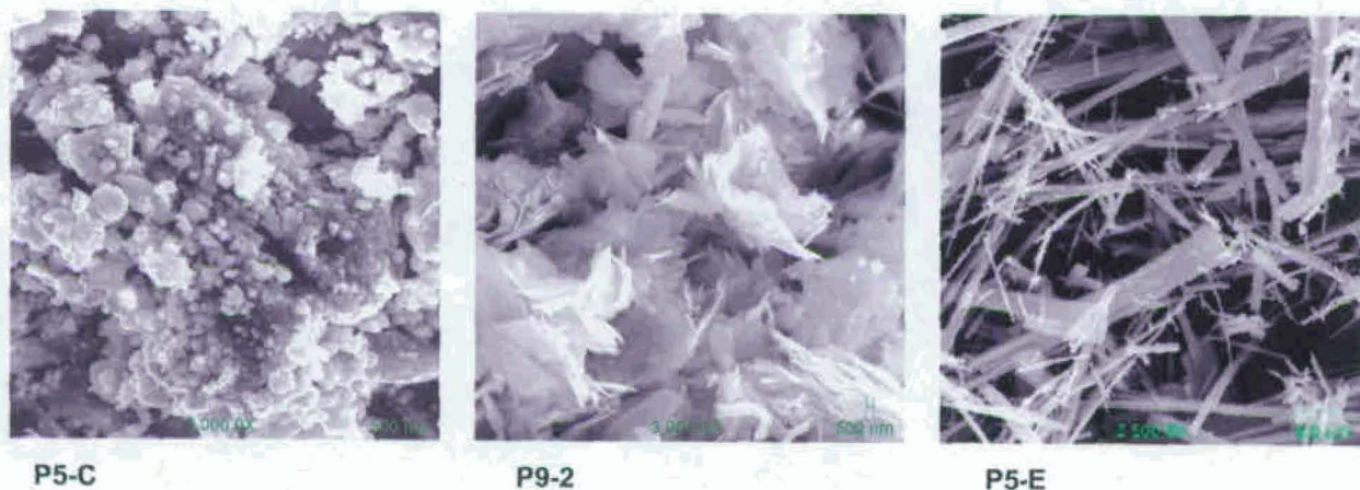
Fig. 6. SEM photographs showing different textures of Bi-based getters; see Table 5 for performance and synthesis details. Occasionally a bladed structure results that is suggestive of layered materials (middle, P9-2). Often, however, the results are granular (left) or needle-like (right).
