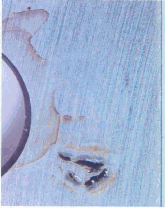
ASW KE0127 X 10 1 Spot Crevice Corrosion
