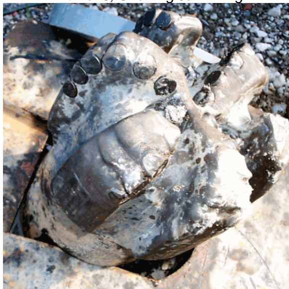
Bit No. 8, Showing Junk Ring
