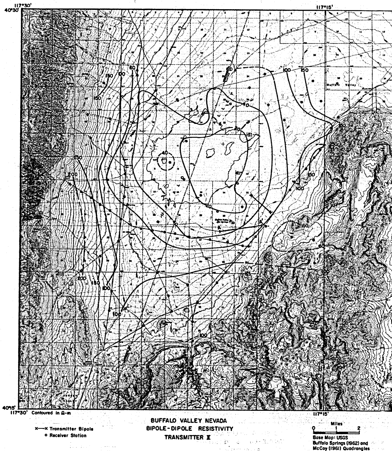
Fig. 15a. Apparent resistivity contours, bipole-dipole survey at Buffalo Valley; current transmitter at location II.
