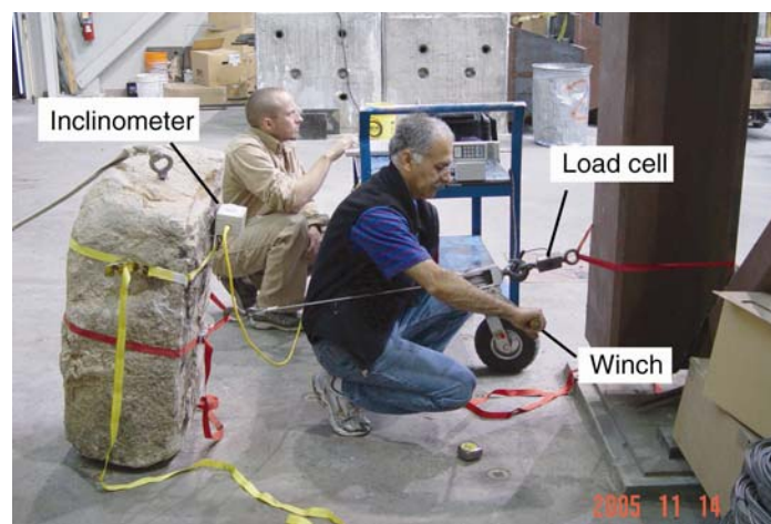
FIGURE 12: Tilt test of one of the stone boulders shaken experimentally.
