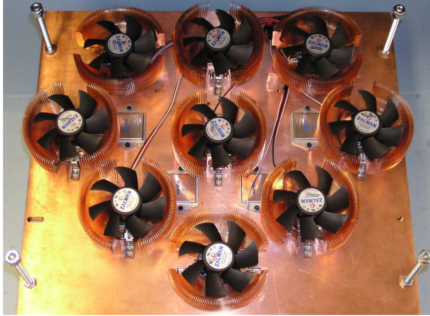
Figure 4-82: Copper plate heat sink with the four power operational amplifiers and nine cooling fans for the 10 kHz FTS.
