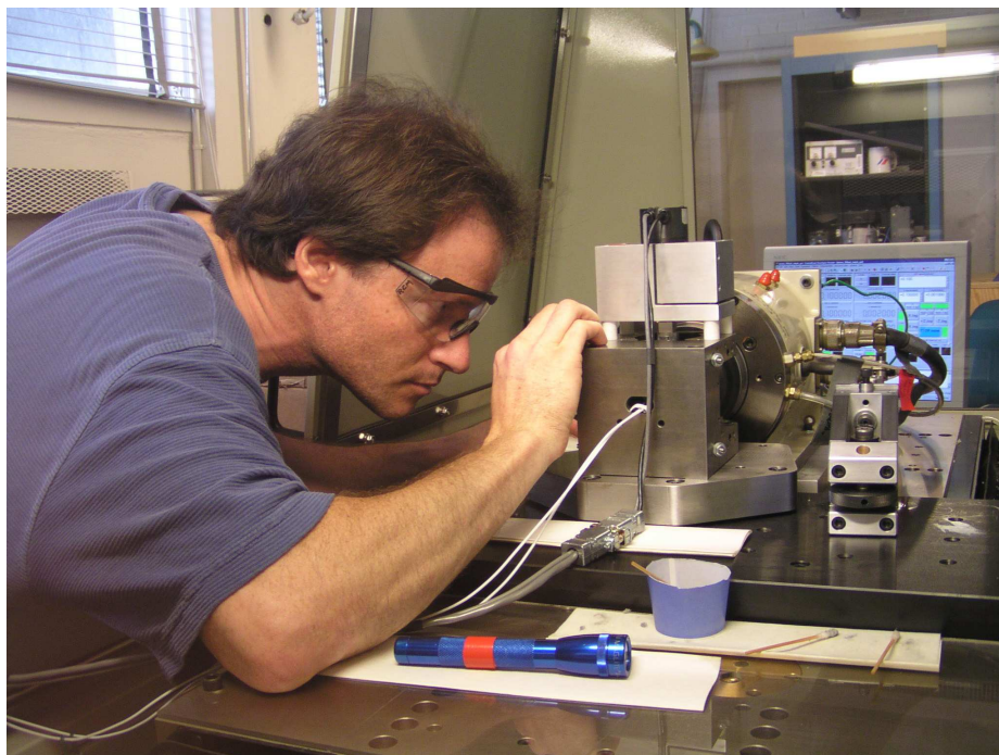
Figure C-14: The author carefully jogging the Z-axis slide of the DTM while establishing initial contact between the diamond tool carried by the 2 kHz FTS and a rotating workpiece. My right hand is holding a magnifying glass that aids observing the first appearance of machining chips on the tool, which indicates contact between the tool and workpiece. My left hand is holding the computer mouse used to select functions in the graphical user interface for the machine, which is visible on the right-side of the figure. Note that the disturbance rejection for the Z-axis slide is sufficient enough for my arm to be resting on the slide while executing a commanded move.
