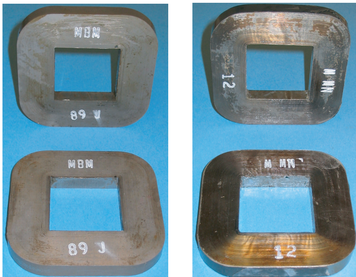
Figure 4-18: Wound-tape core blanks for the rotor. Conventional Ni-Fe (left), and nanocrystalline amorphous Ni-Fe (right). Each core blank can provide four rotor cores.
