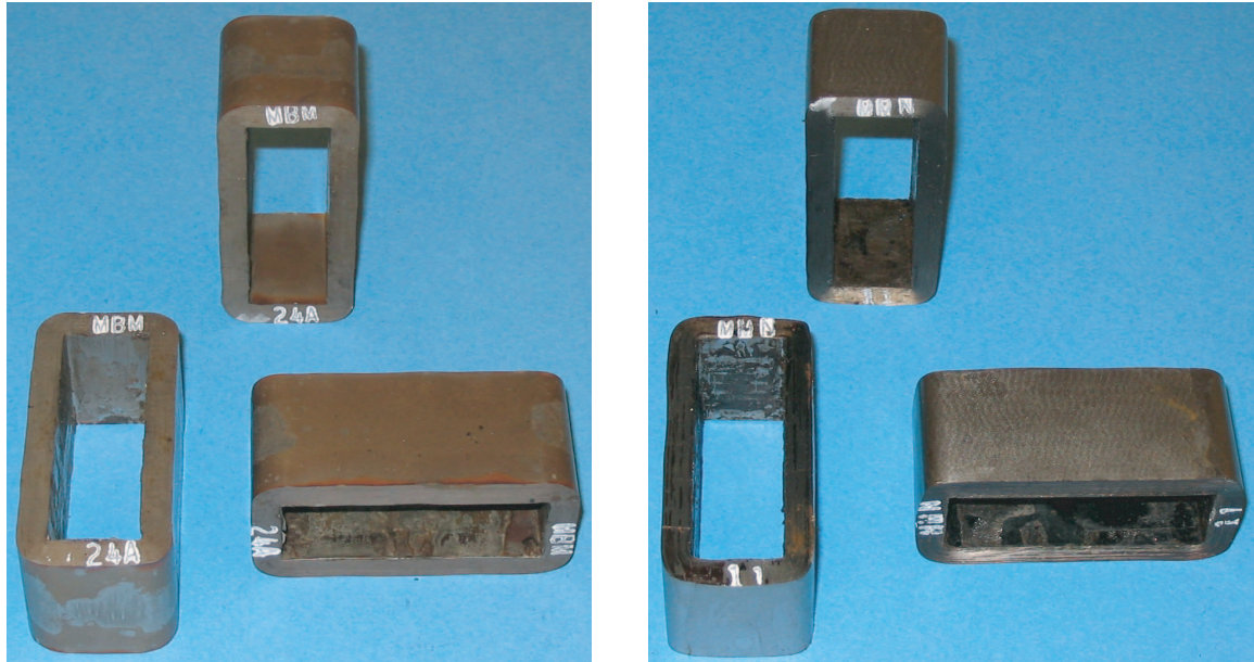
Figure 4-19: Wound-tape core blanks for the stators. Conventional Ni-Fe (left), and nanocrystalline amorphous Ni-Fe (right). Each core blank can provide two stator cores.
