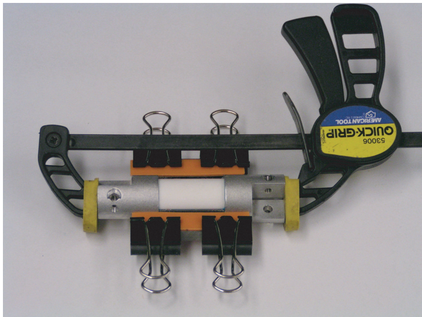
Figure 4-25: Clamping of the full assembly of the rotor core, ceramic stiffeners, and flexure hubs for the 10 kHz FTS, during cure of the epoxy adhesive.
