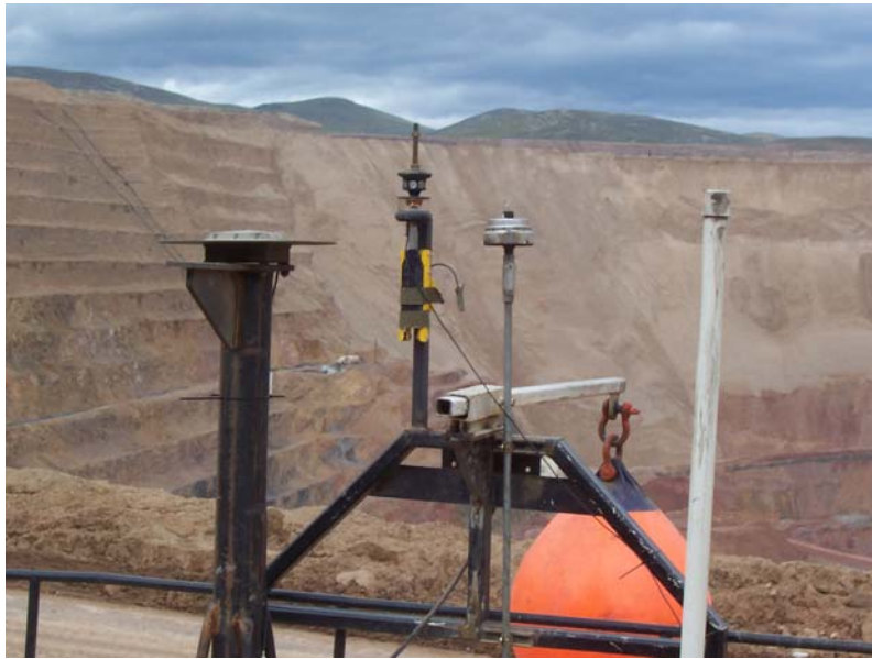
Figure 22: Mounting positions of the GPS antenna and the ATS prism.
