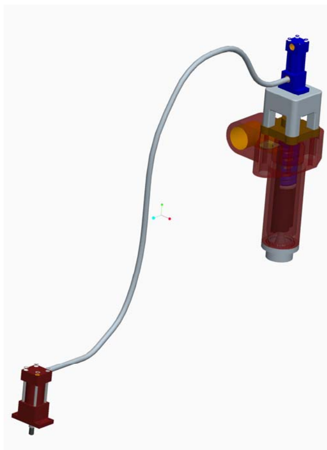
Figure 50 Hydraulically actuated mechanical fuel injection valve system
