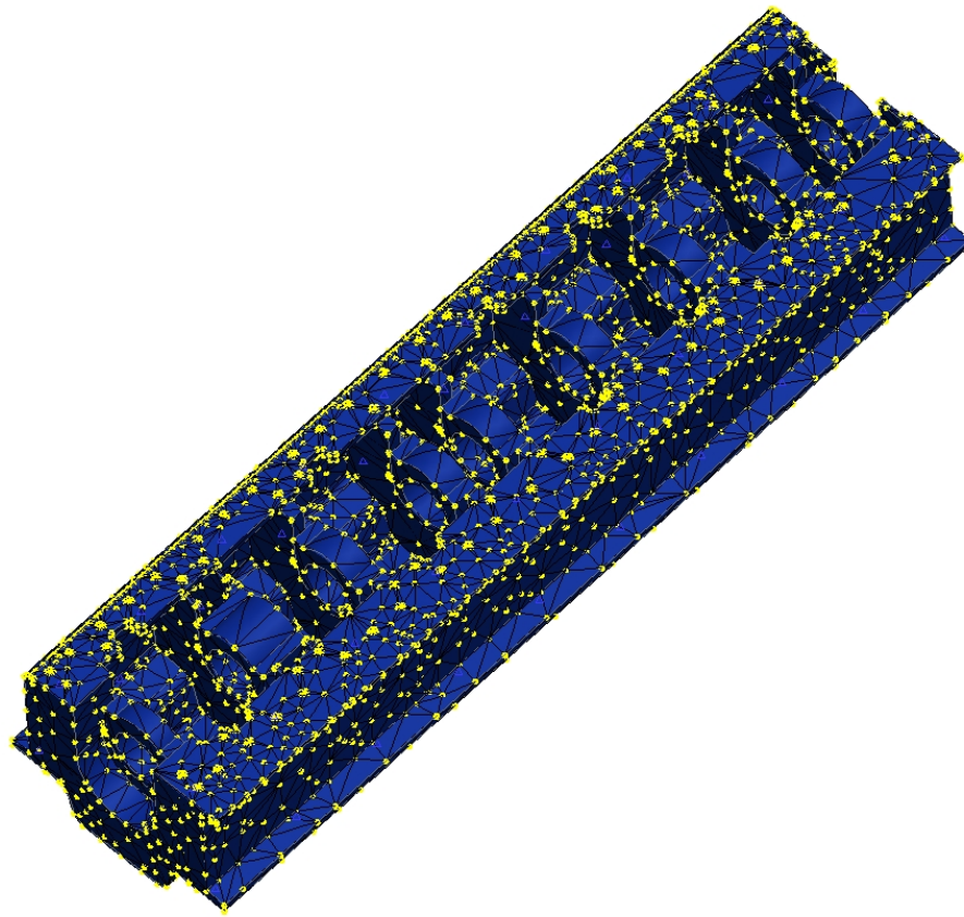
Figure 36 Mesh of the simplified TLA-6 crankcase
