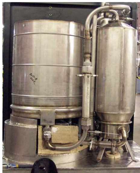
Natural Gas Fueled SOFC System In Operation at VPS
