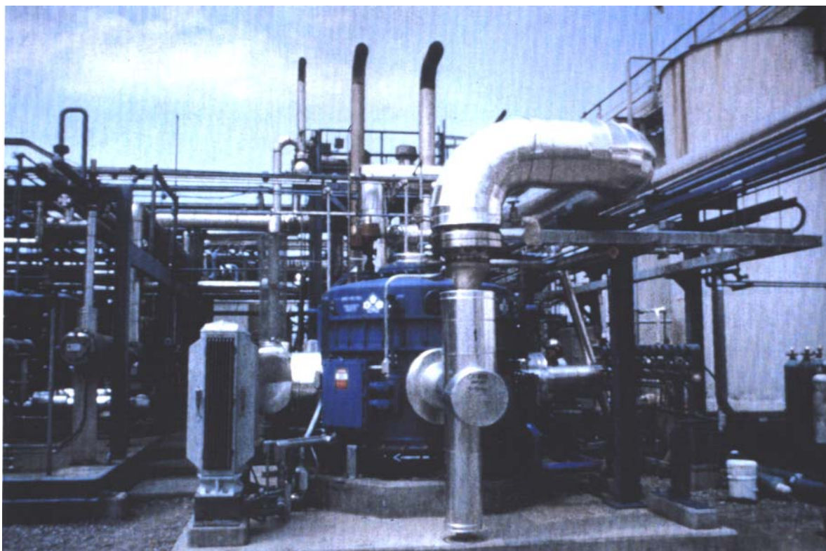
Figure 1-2. 20 kW Carbonate Fuel Cell Test at the LGTI Gasification Facility Completed in 1992
