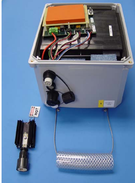
Figure II-16: Battery power enclosure with discharger
