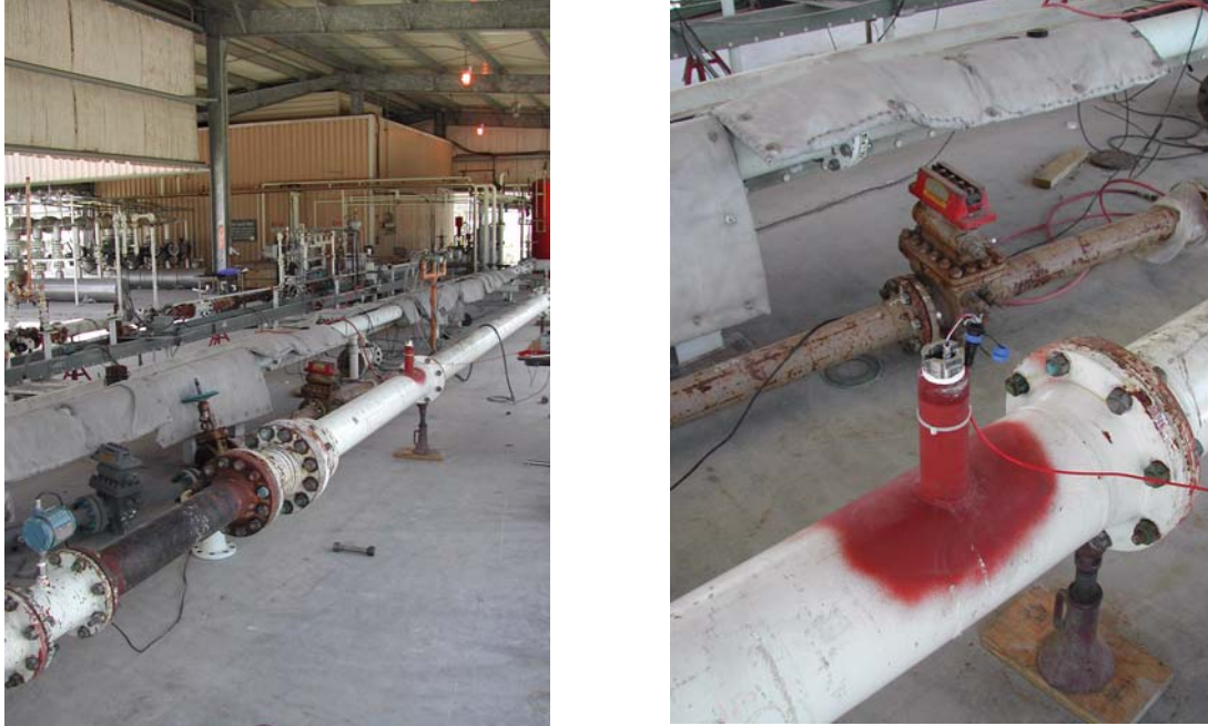
Figure II-24: SwRI Metering Test-Loop Calibration Setup
