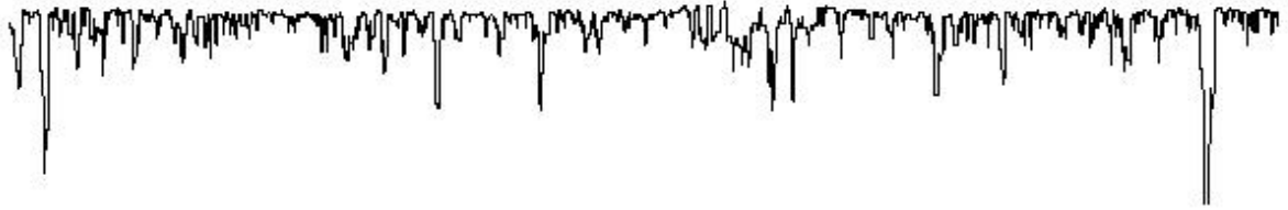
Figure 1-2: Typical plateau honed profile
