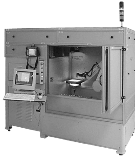
Figure 1-5: Typical laser texturing machinery (from Control Micro Systems, Inc.)
