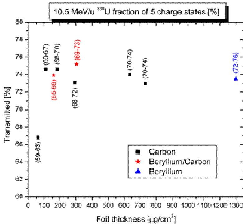
Figure 2: Sum of highest four charge state fractions (which could be transmitted in the RIA driver) emerging from different foil types and thicknesses as measured with an 85 MeV/u Uranium beam at GSI.
