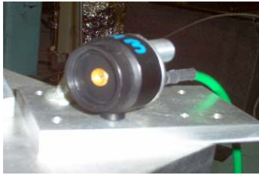
Figure 3: The photodiode detector, positioned behind the shutter box.
