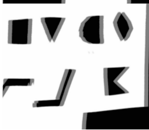
Image 2: 80mm scan of template is blurry and stretched because of offsets in count time and shutter time.
