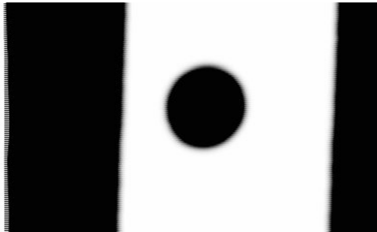
Image 3: Part of 80mm scan of knife edges. This image has near-perfect count time and a shutter time offset of only one pixel (see Table 1).
