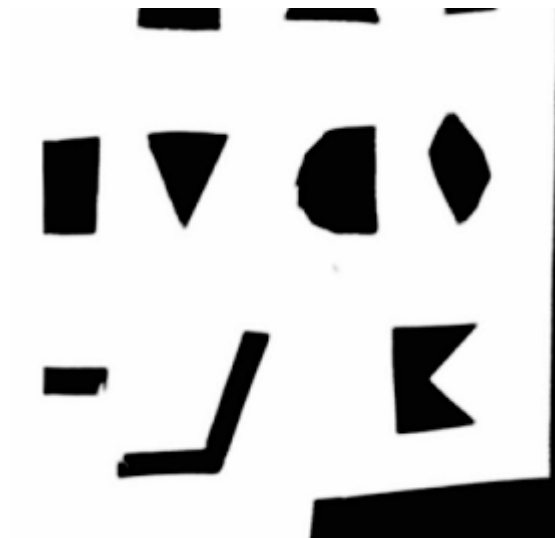
Image 4: 80mm scan of stencil, repeated using new parameters from knife edge scan (see Table 1).
