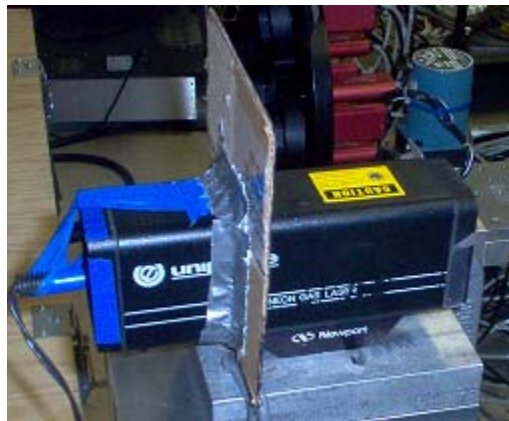
Figure 1: The class II He Ne laser was positioned in front of the stage (below).
