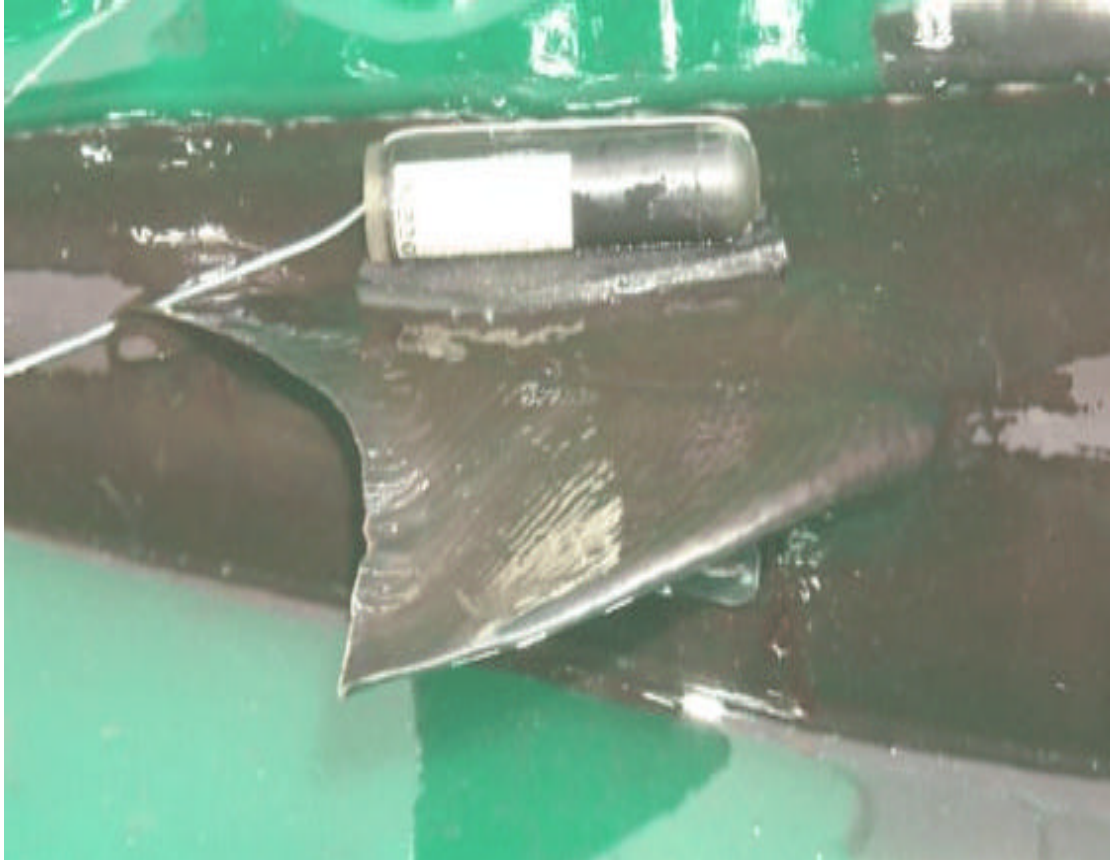
Figure 2. Placement of a Combined Acoustic Radio Tag (CART) on a white sturgeon.
