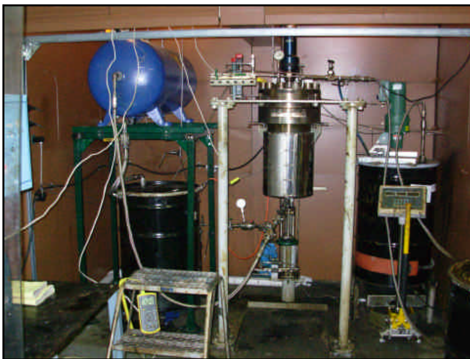
Figure 1. Modified reactor system for carrying out digestion.
