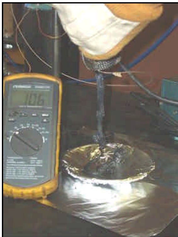
Figure 79. Extrusion test with a 110 °C softening point pitch extruded at approximately 106 °C.
