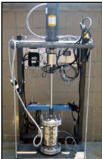
Figure 83. Test stand including reactor designed to enhance anisotropy of coke.
