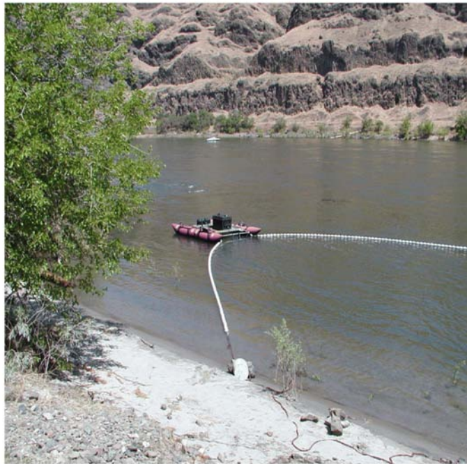
Figure 2. Floating PIT-tag detector antenna (top) and unit deployed in the free-flowing Snake River, 2003.
