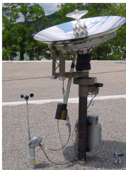
Fig. 44. Solar collector installed above the bioreactor.
