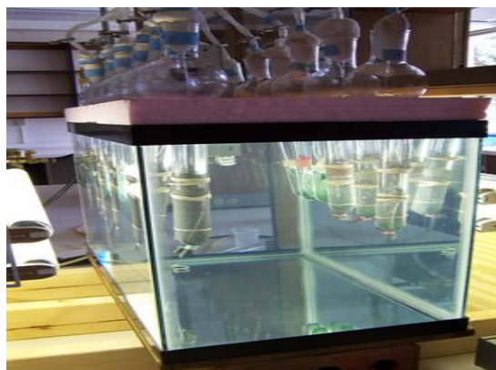
Fig. 18. General view of the photoreactor with tubes coated with different screening mesh.
