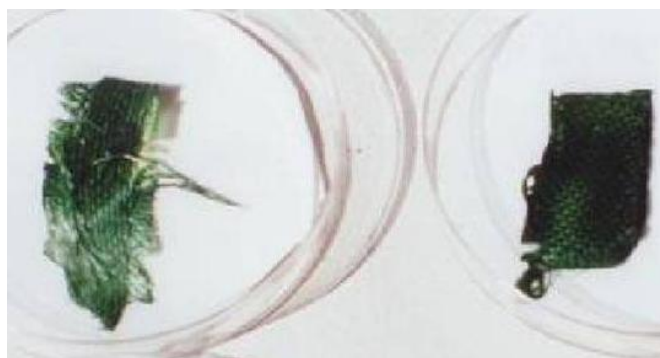
Fig. 30. Omnisil coupons are shown untreated (left) and treated with \text{Ca}^{2+} (right).
