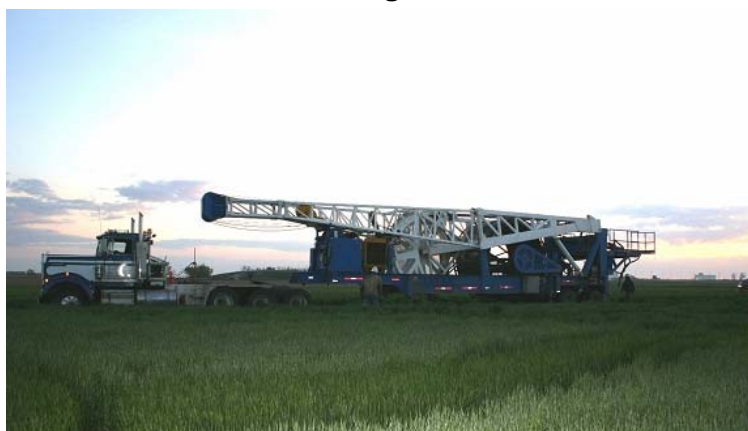
Figure 5 - CT Rig in Trailering Position; Rig Trailer with Dimensions of 50' in Length, 12' Wide and 15' in Height
