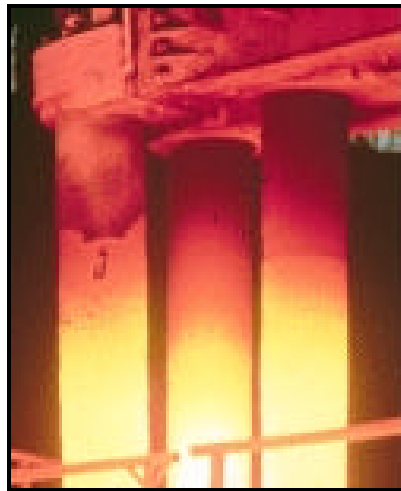
Figure 5. Close-up of arc furnace electrodes, operating at 3000 °C. Courtesy GrafTech International.
