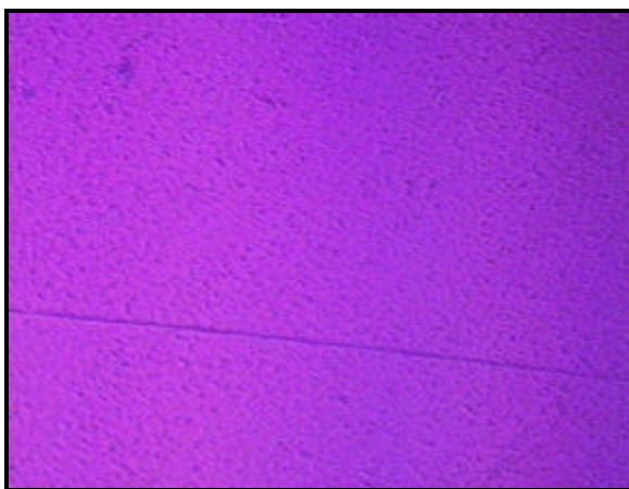
Figure 96. Optical Micrograph of Pitch Sample with Recovered RCO at 400 °C, 500 psig Cold Hydrogen, 5/1 Solvent-to-Coal Ratio and One Hour Reaction Time.
