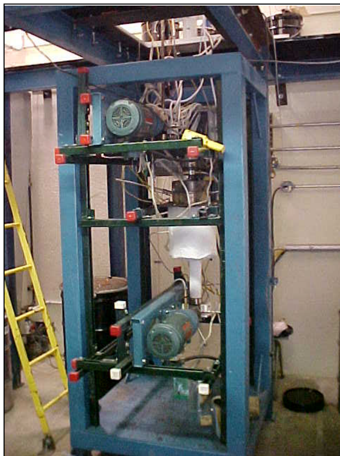
Figure 30. Lower Level Reactor Used to Chemically Digest Coal.
