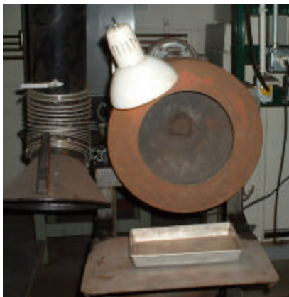
Figure 3.1 Laboratory scale pelletizing drum with overall diameter 40.6 cm (16 in), mouth diameter 25.4 cm (10 in) and depth 17.8 cm (7in) rotating in a counter-clock wise direction at 35 rpm.
