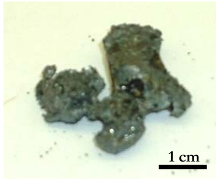
Figure 4.5 The transition direct reduced iron produced at furnace temperature 1425 °C and furnace residence time 28 min. Its apparent density is lower than pig iron nuggets, and higher than DRI. This is due to the reduced amount of porosity, and partial slag separation, and higher metallization.
