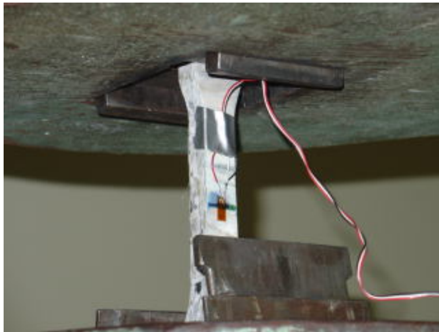
Figure 0-17 Close up of the Tension test setup
