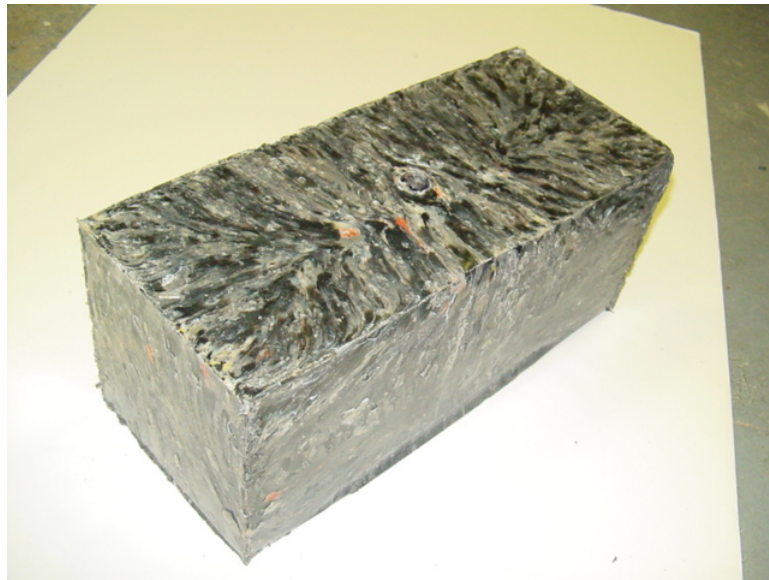
Figure 4-10 Final offset block with recycled ABS blends
