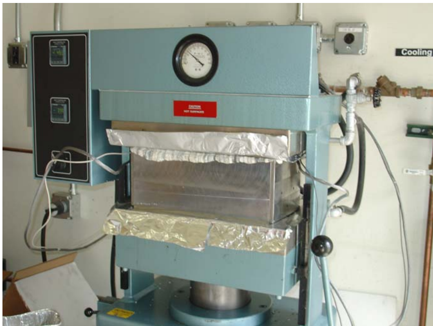
Figure 0-11 Mold compressed under pressure and temperature
