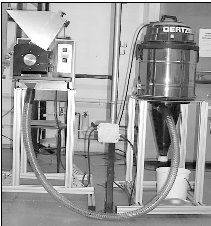
Figure 25: Fritsch cutting mill no. LC-136 used to shred waste EOL Plastic
