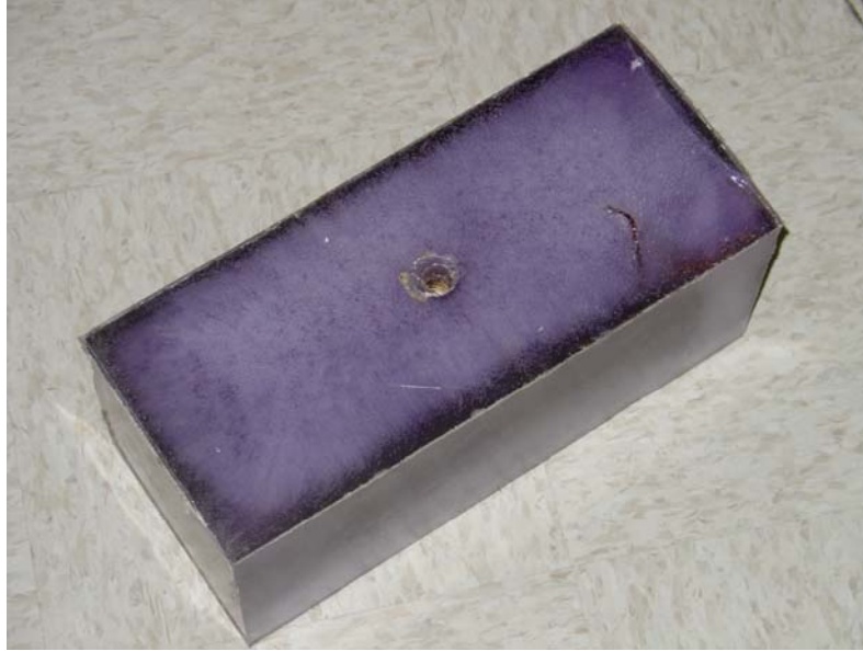
Figure 4-11 Final offset block with recycled PC blends
