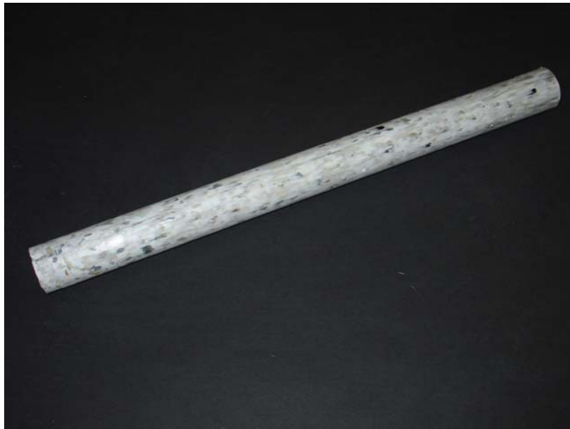
Figure 0-7 Appreciable surface finish and blending in dowel, with increase in process time
