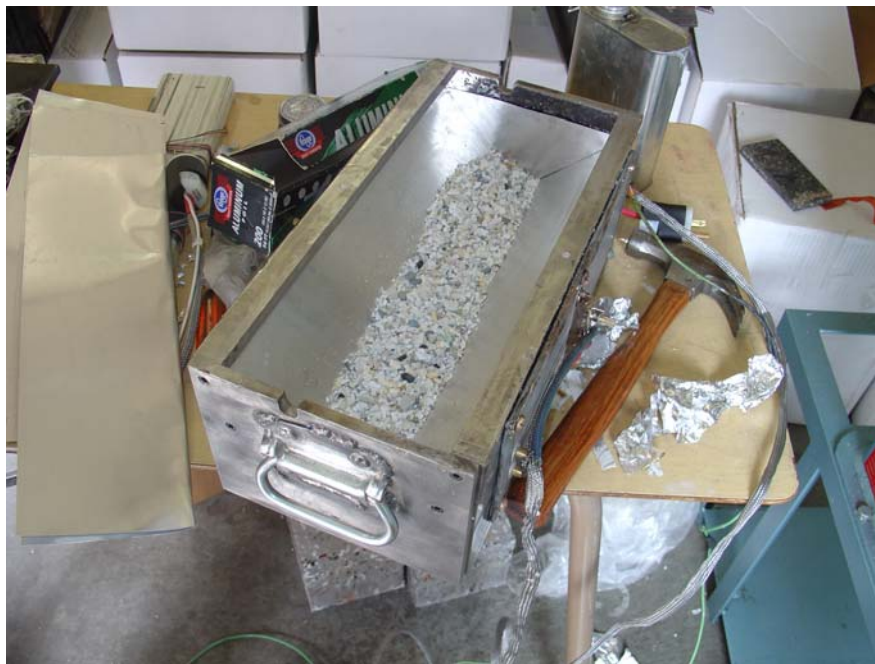
Figure 0-9 Angle mold being filled with ABS resin
