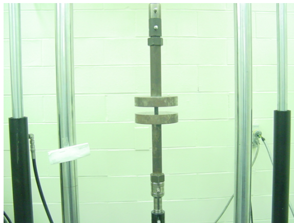
Figure 0-7 Compression test set up for ABS specimen
