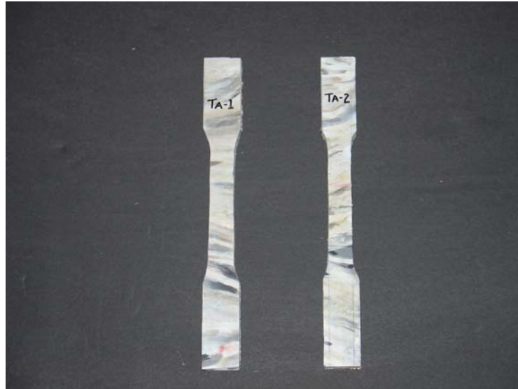
Figure 0-15 Tension coupons cut from angle
