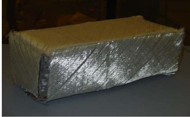
Figure 4-13 Glass fabric wrapped around wooden core with premolded polymer plates
