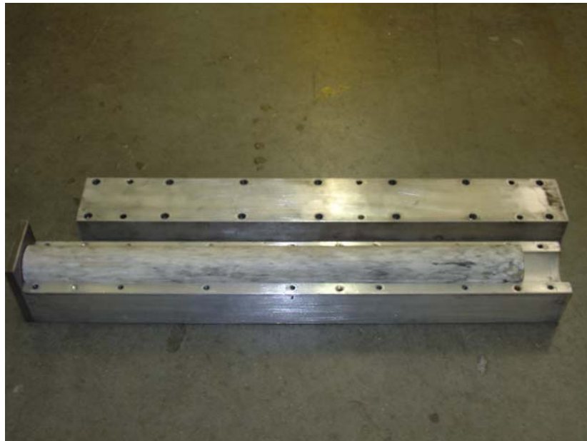
Figure 0-5 Mold with dowel bar after first process cycle
