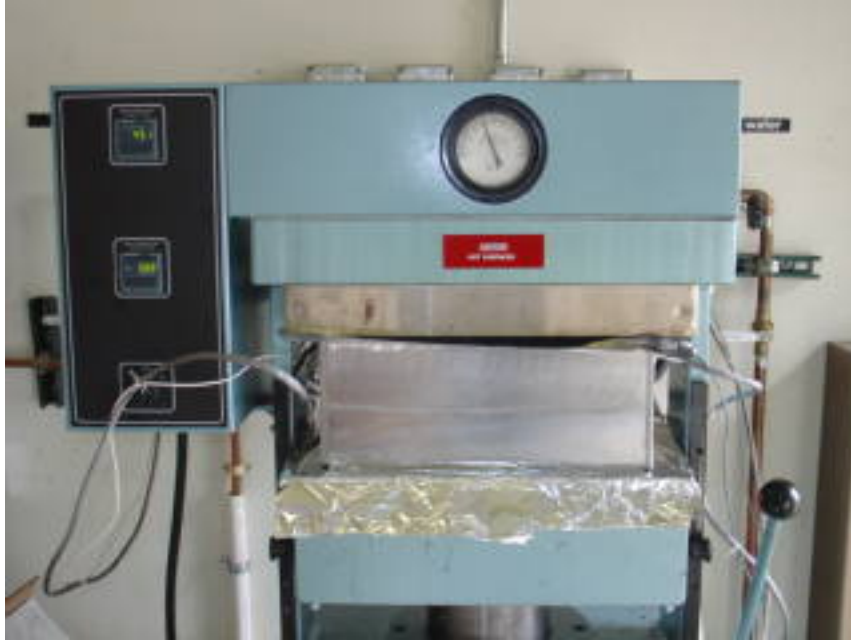
Figure 0-12 Mold being cooled in the compression press under dead load
