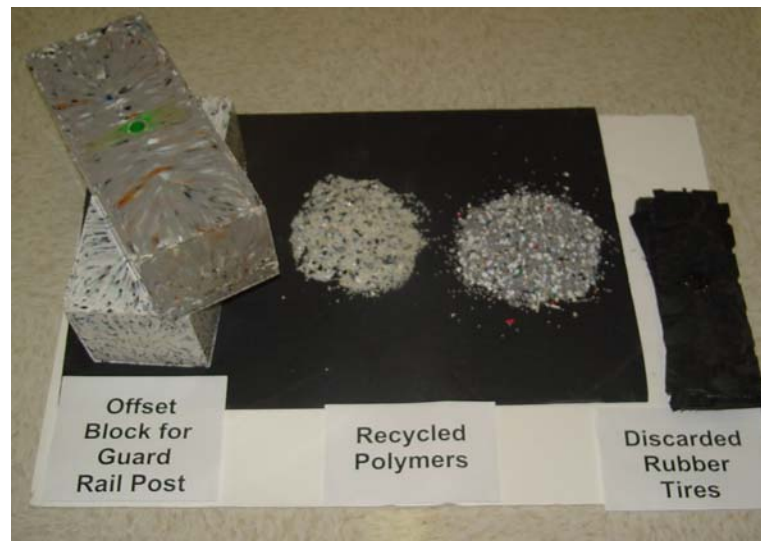
Figure 4-1 Guardrail offset blocks and constituents
