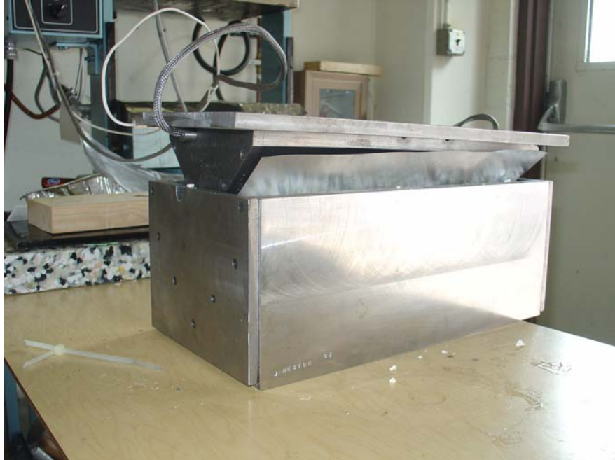
Figure 0-10 Angle mold filled with ABS resin reinforced with glass fabric
