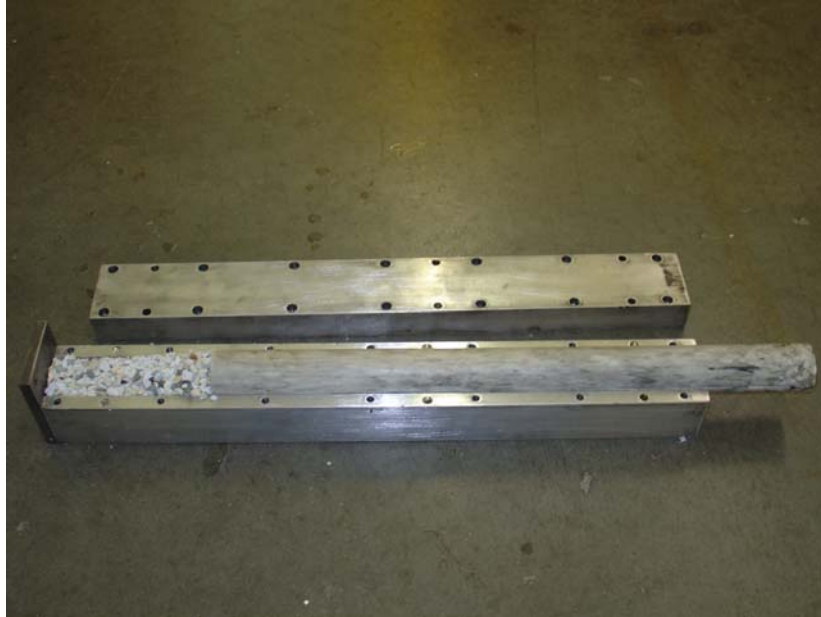
Figure 0-6 Mold with additional pellets and premolded bar for following cycles
