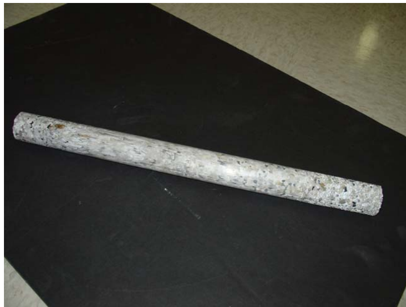
Figure 0-4 Unblended resin pellets in the dowel due to inadequate heat transfer
