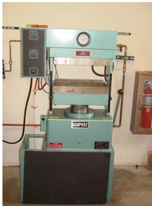
Figure 4-4 PHI Compression molding press with thermostat controls and temperature displays
