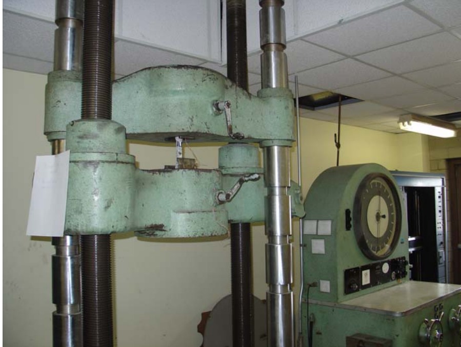
Figure 0-16 Tension test specimen in Baldwin machine
