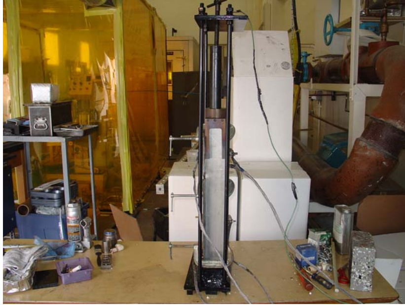
Figure 0-3 Experimental mold setup for dowel bar manufacture
