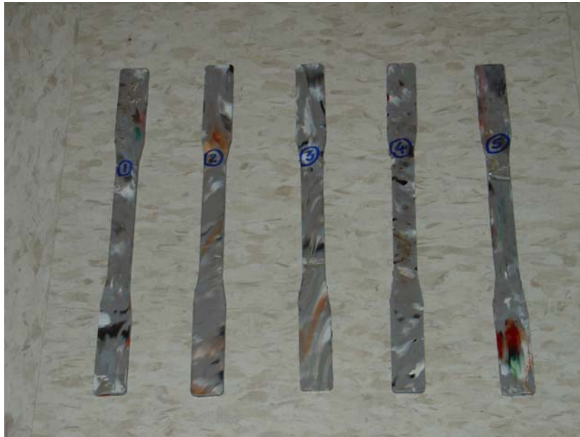
Figure 0-2 Compression-molded tension test samples
