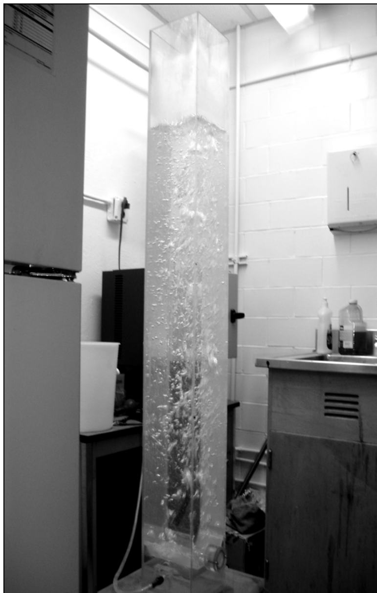
Figure 26: Experimental Rig used in Froth Floatation of EOL Plastic
