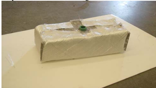
Figure 4-12 Core module wrapped with glass fabric
