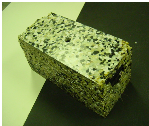
Figure 4-8 Unblended pellets on the block surface
