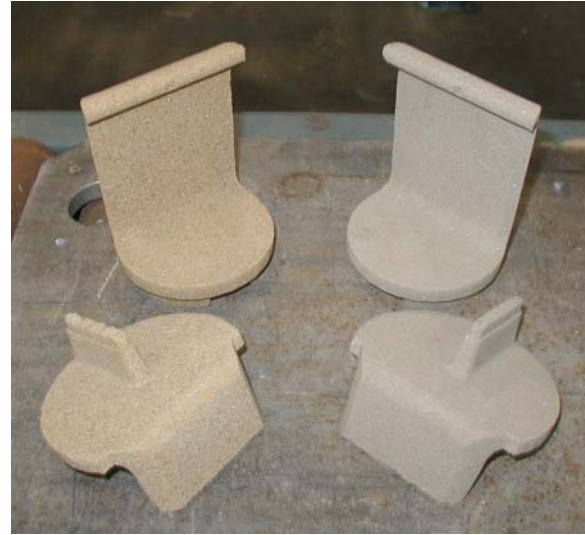
Fig. 5 Fabricated inserts with GFN 47 (left) and GFN 97 (right).
