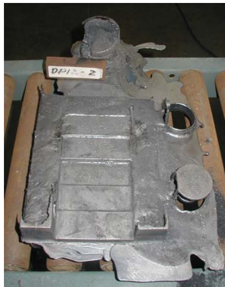
Fig. 21 DPI2-2 after shake-out. Note complete filling of all plates.
