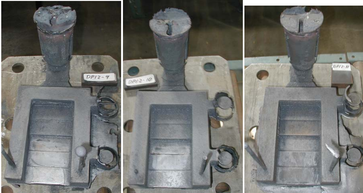
Fig. 44 View of the castings after shake out. Left DPI2-9, middle DPI2-10, right DPI2-A. Note the shape of the metal on top of the top insert, especially the opening created by the handle piece.
