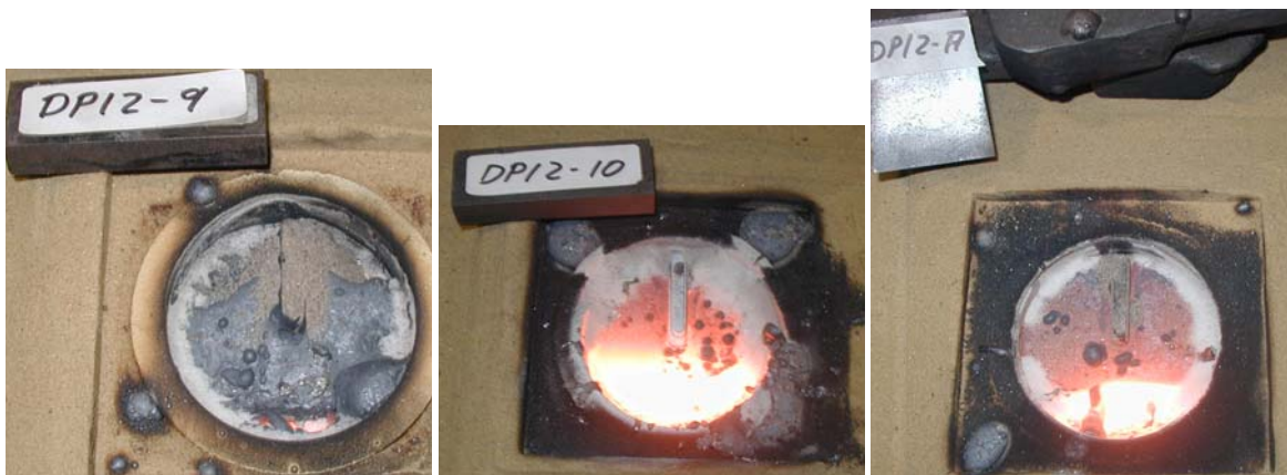
Fig. 43 View of the top inserts after pouring. All inserts retained their shape.
