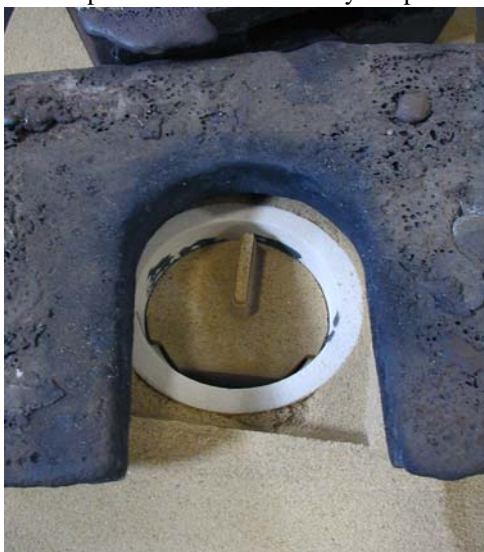
Fig. 34 Left: top insert glued into position by core paste, right: DPI2-4 minutes after pouring with top insert slowly disintegrating
