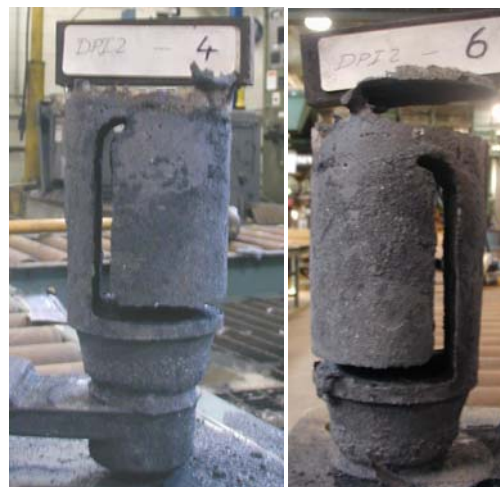
Fig. 36 Side view of container DPI2-4 and DPI2-6 after shake out.
