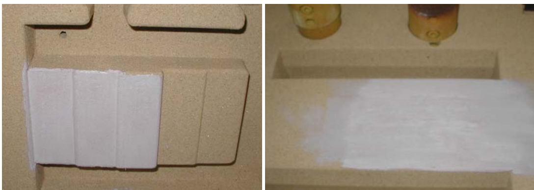
Fig. 49 Coated cope (left) and drag (right) of molds for the 5 th heat.
