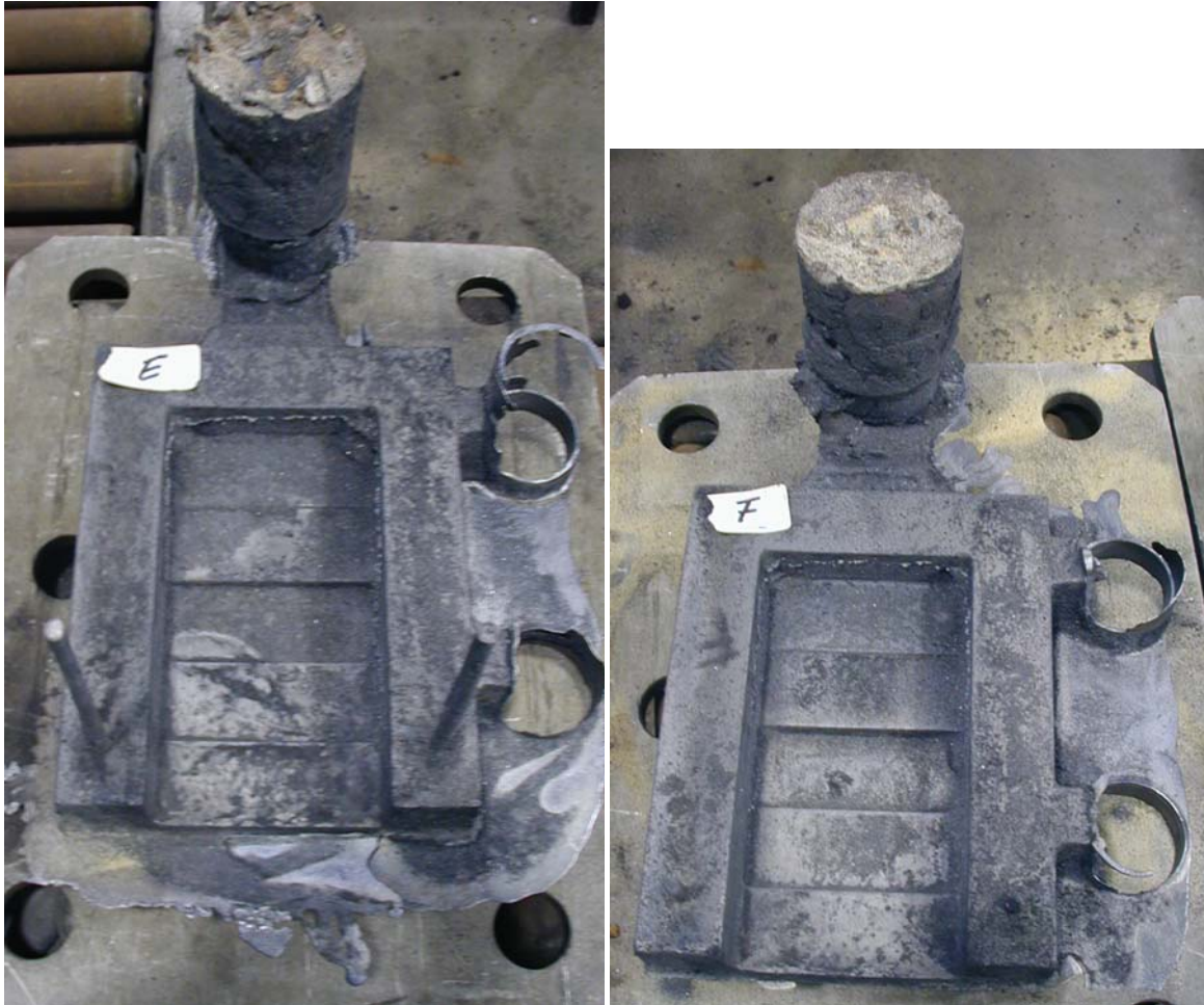
Fig. 54 Castings DPI2-E and DPI2-F after shake-out.
