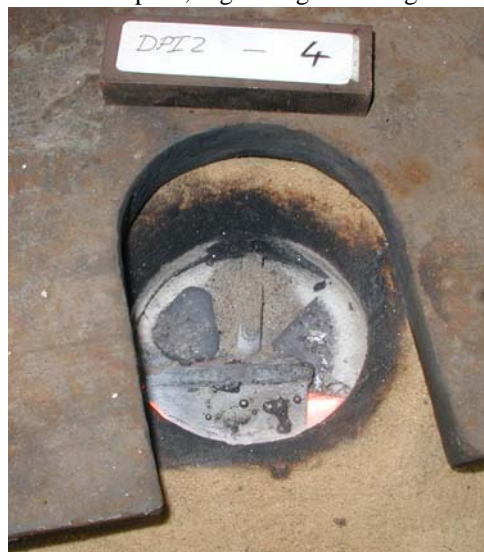
Fig. 34 Left: top insert glued into position by core paste, right: DPI2-4 minutes after pouring with top insert slowly disintegrating
