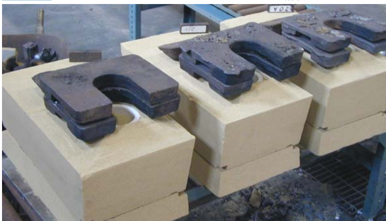
Fig. 15 Molds ready to be poured (l DPI2-1, mid. DPI2-2, r DPI2-3).
