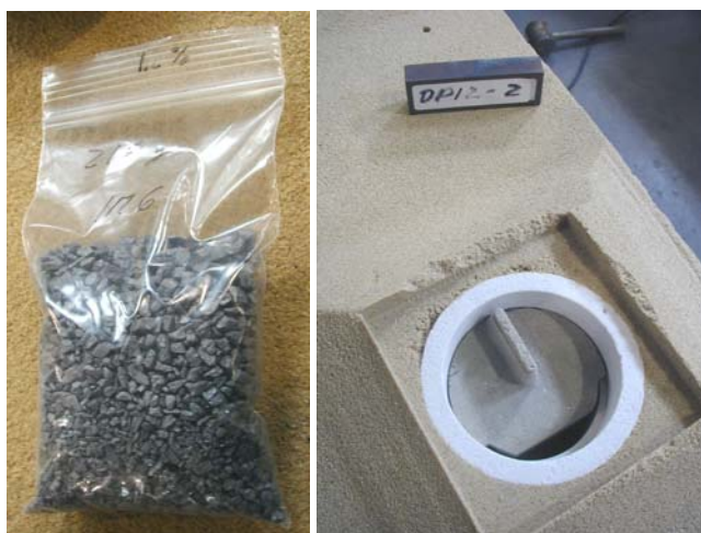
Fig. 11 Detail of alloy bag (left) and top view of completed sleeve (right).
