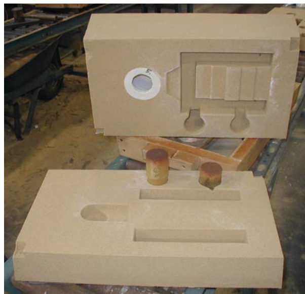
Fig. 8 Open mold halves with DPI2 sleeve and spectrometer inserts in place.
