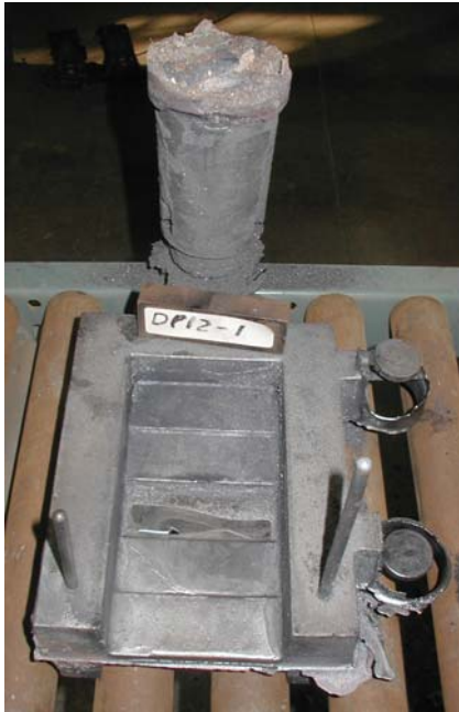
Fig. 19 DPI2-1 after shake-out. Note cold shot at 2mm plate.
