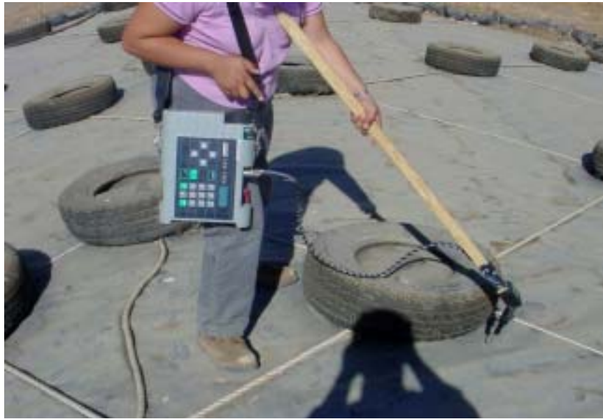
Image 3-6. Surface emission monitoring with the TVA 1000.
