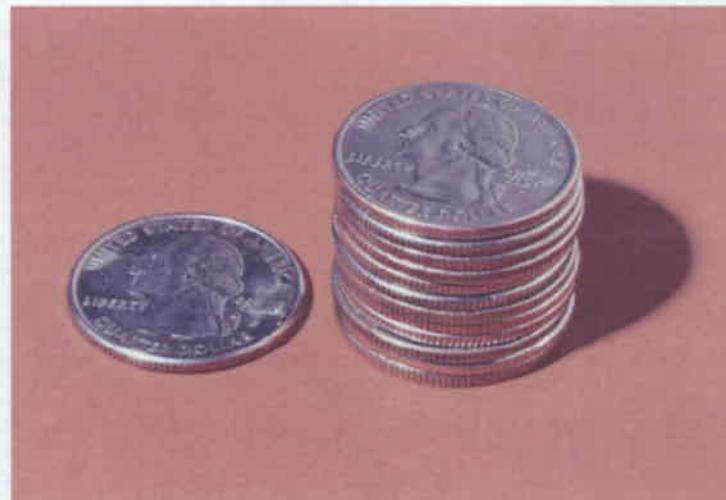
**16,000 to 160,000 years to penetrate the thickness of one U.S. quarter for a corrosion rate of 0.1 to 0.01  $\mu\text{m}/\text{yr}$**
