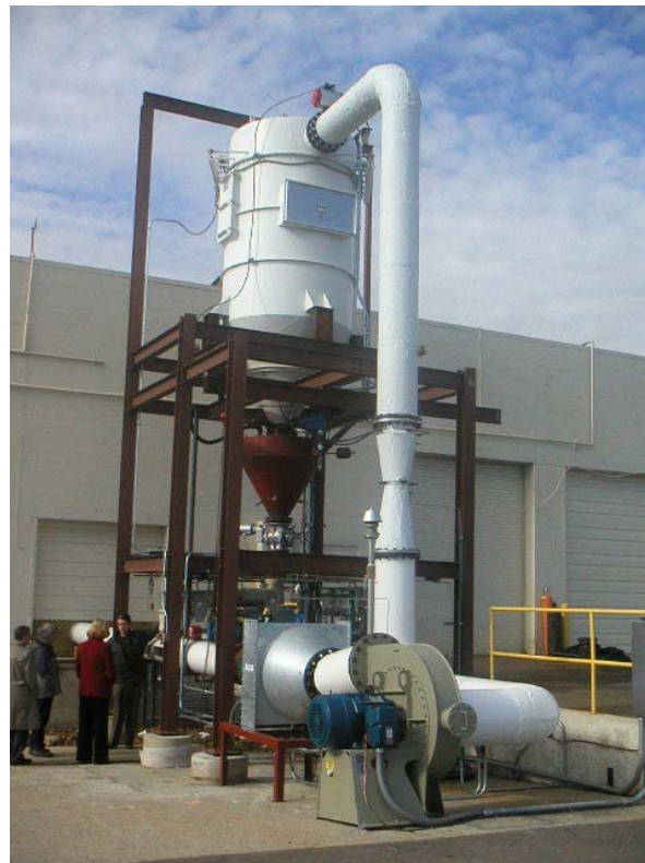
Figure 6. EPRI & Airflow Sciences pulverized coal and air supply system
