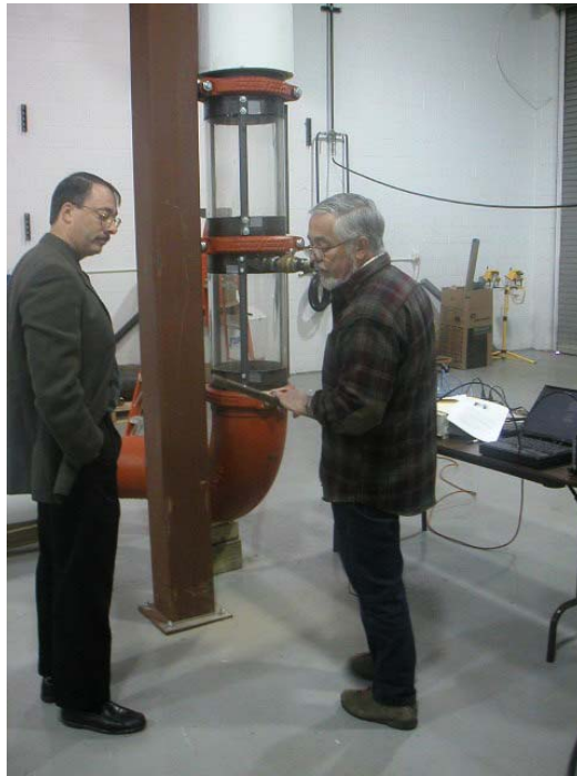
Figure 7. Transparent coal and air test section
