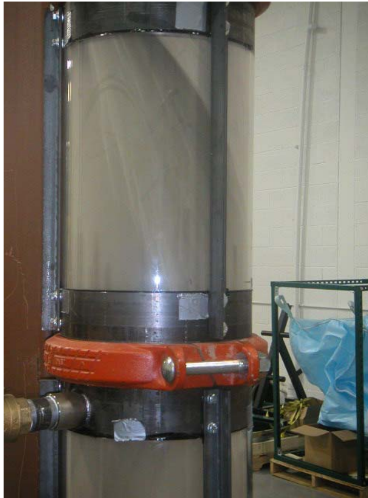
Figure 9. Test section with silicon particles and air, swirl induced by offset elbows upstream
