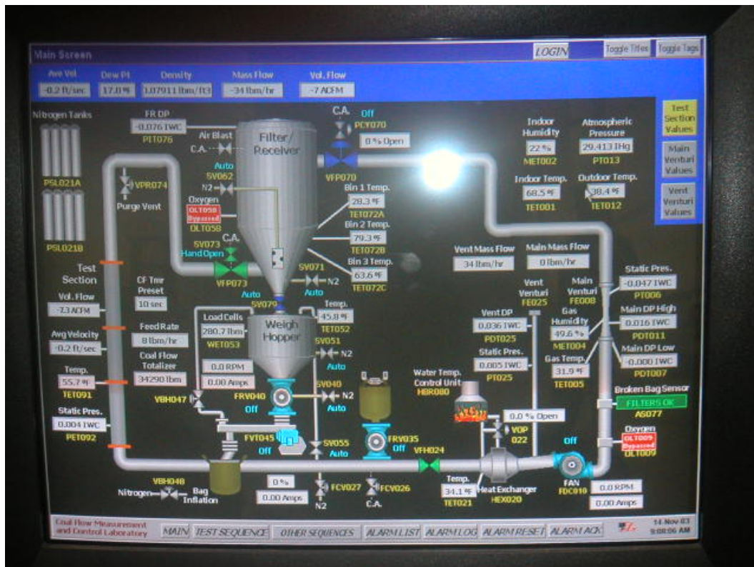
Figure 8. CRT display of Coal Flow Loop schematic, instrumentation and controls
