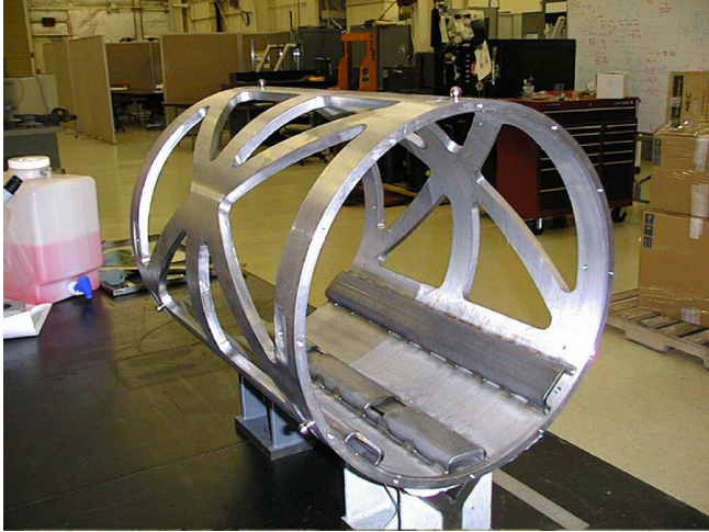
FIG. 7: The Livermore space frame held the entire three-BPM assembly rigid. The first vibrational mode was at 200 Hz.
