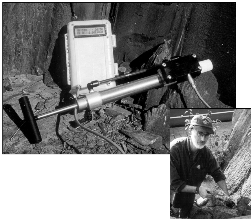
Figure 17: The hand-held air permeameter for fractures christened “TinyPerm.”
