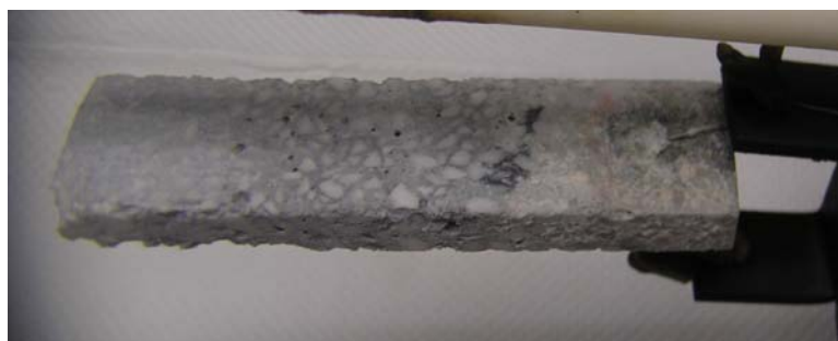
Fig. 4.20. Candidate high-MgO alternative backup lining material after smelt immersion testing.
