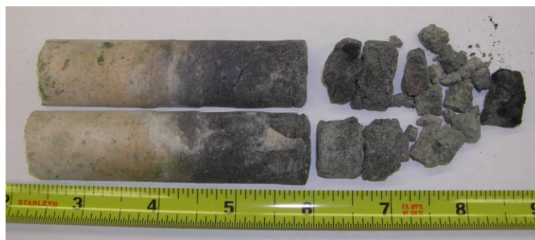
Fig. 4.19. Backup lining core sample removed from New Bern gasifier showing crumbled hot face and discoloration due to smelt penetration/reaction.
