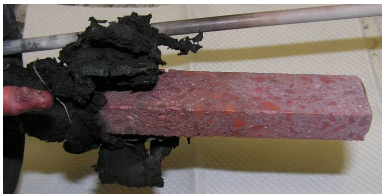
Fig. 4.21. ORNL-developed alkali-aluminate backup lining material after smelt immersion testing. Note the extent of degradation of the metallic holder held in proximity of the molten smelt.
