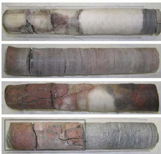
Fig. 4.2. Images of core-drilled specimens. From top to bottom: primary fusion-cast alumina lining material, fusion-cast magnesia-alumina spinel test block, alternative fusion-cast alumina test block, and bonded magnesia-alumina spinel test block (outlined on left).
