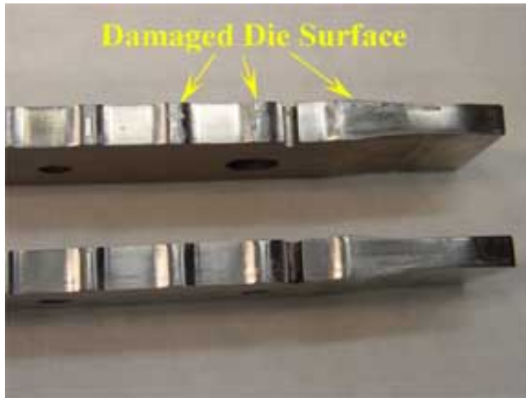
(a) The damaged surface of the inlet die channel
