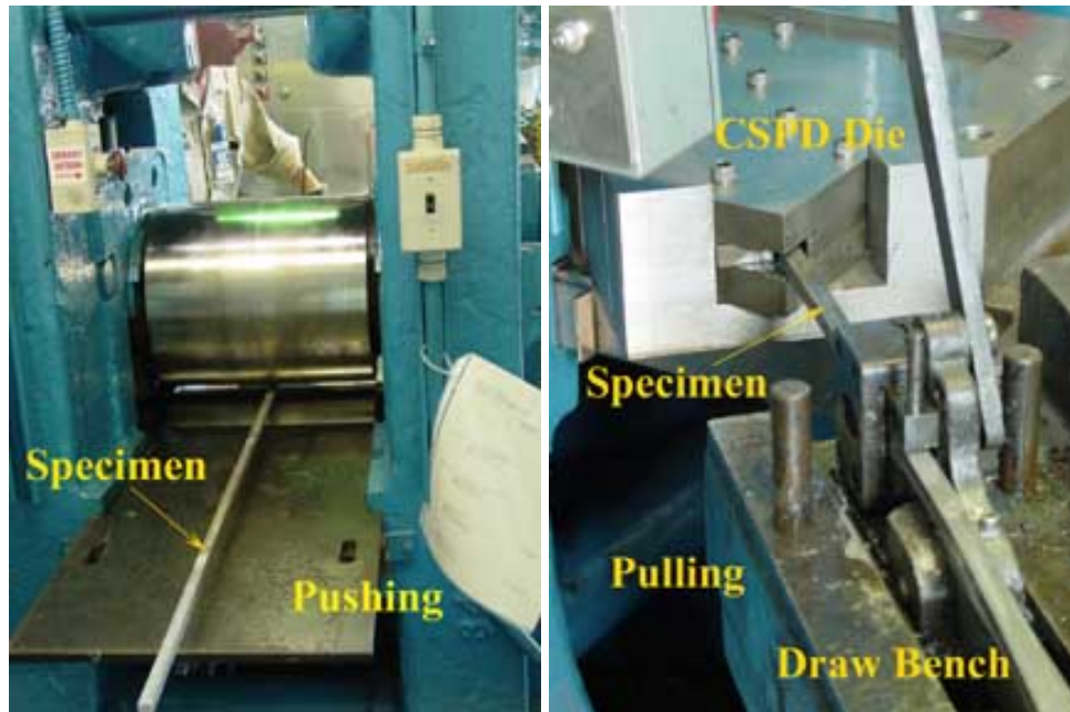
Figure 3.16: A long AA6061 specimen being pushed and pulled during CSPD. Three passes were made using the roll+draw setup
