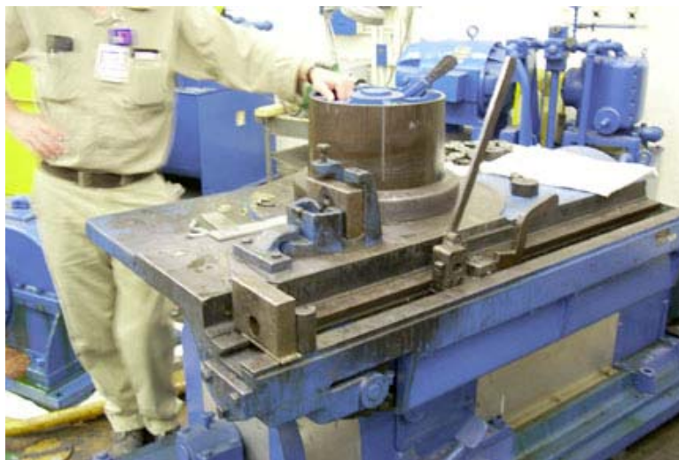
Figure 3.14: The draw bench used to pull the extruded bar during CSPD
