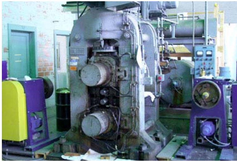
Figure 3.13: An 80 horsepower United Mill used to push metal bars during CSPD.
