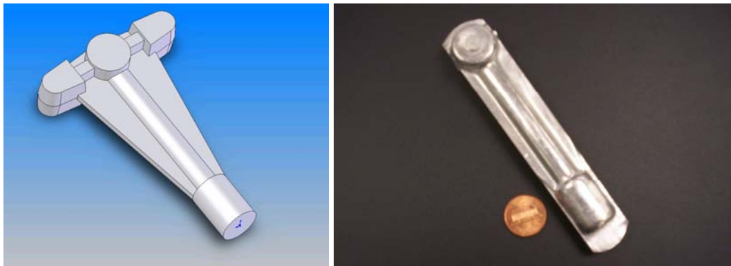
Figure 4.18: Solid model and a trimmed forging of the part used for making fatigue samples
