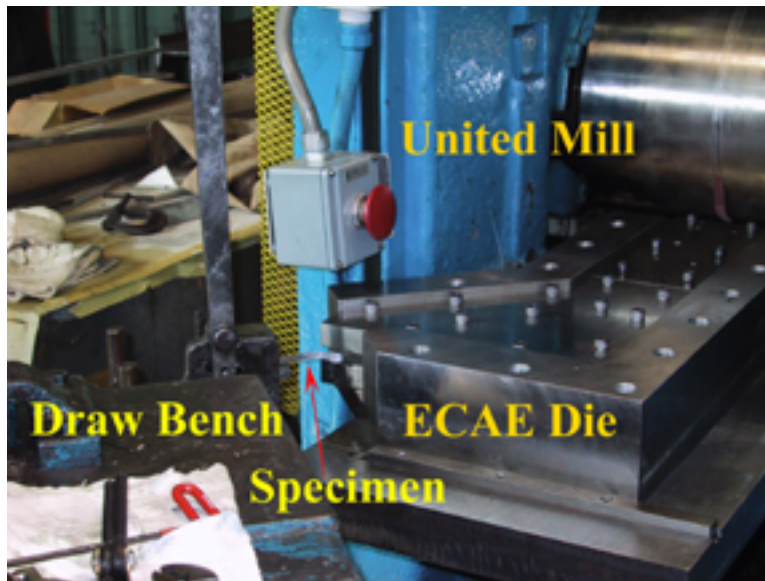
Figure 3.15: The setup of the United mill, the draw bench, and the ECAE/P die for CSPD
