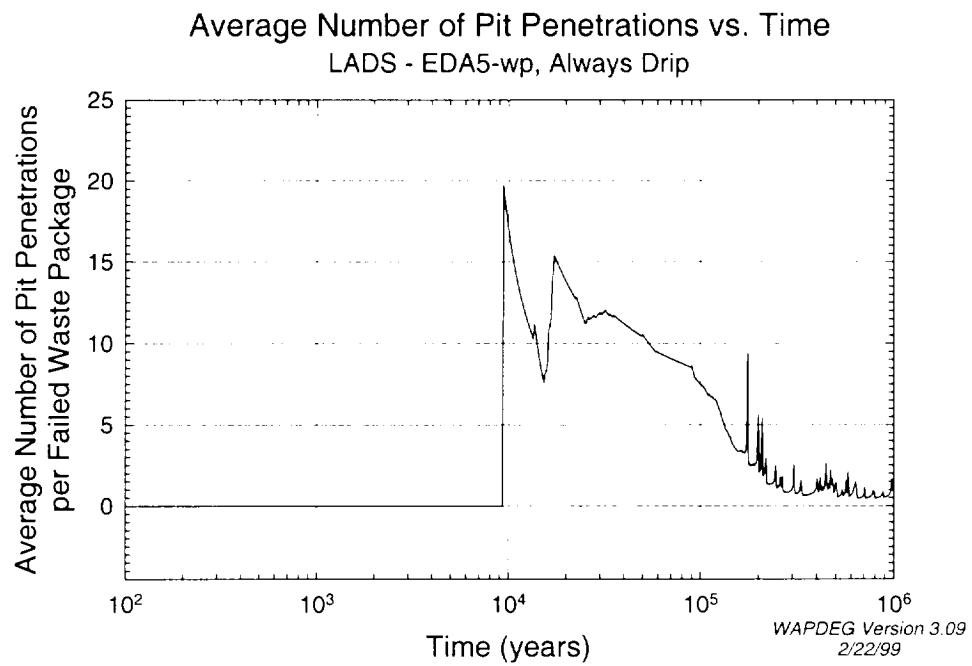
The first breach curve for the waste package and the average number of pit and patch penetrations per failed waste package curves are also represented in the RIP input table, NE1a5s5EDA5-wp.rip.
